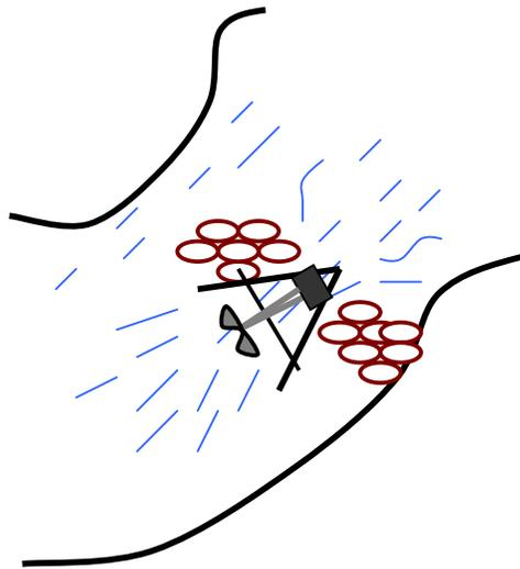
Figure 11 - Schematic figure 'lying' pico-hydro unit in River
