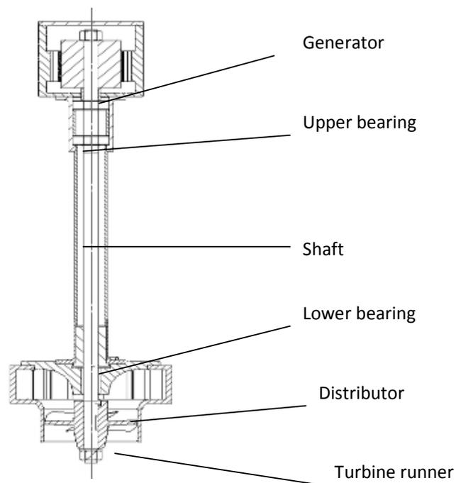
Figure 3 - Schematic picture of low-head propeller type pico-hydropower unit (Entec, 2000)
