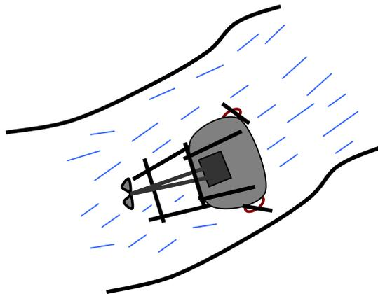
Figure 13 - Schematic figure pico-hydro on raft-like structure
