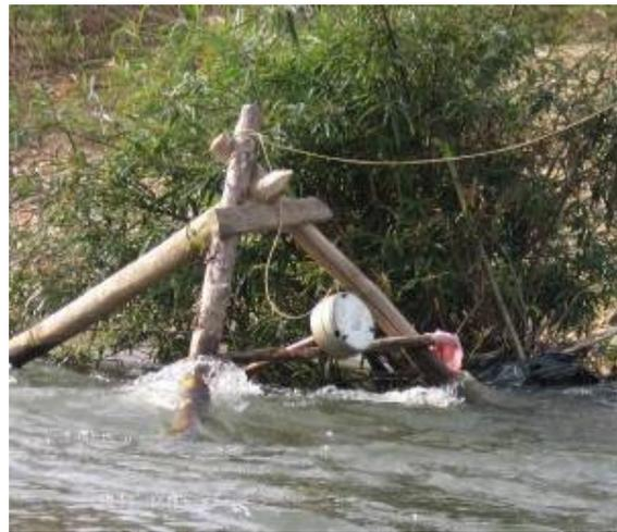
Figure 12 - 'Lying' pico-hydropower unit in Nam Muan river, Bolikamxay
