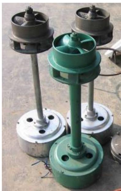
Figure 1 - Low-head propeller pico-hydro units
