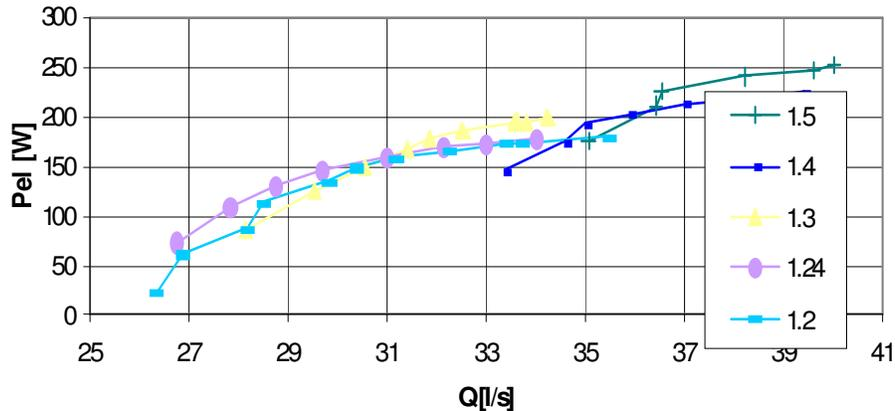
Figure 4 - Power output ( $P_{ei}$ ) variation for a low-head propeller pico-hydropower turbine with varying flow ( $Q$ ) and a different constant heads (colored lines) (Entec, 2000)
