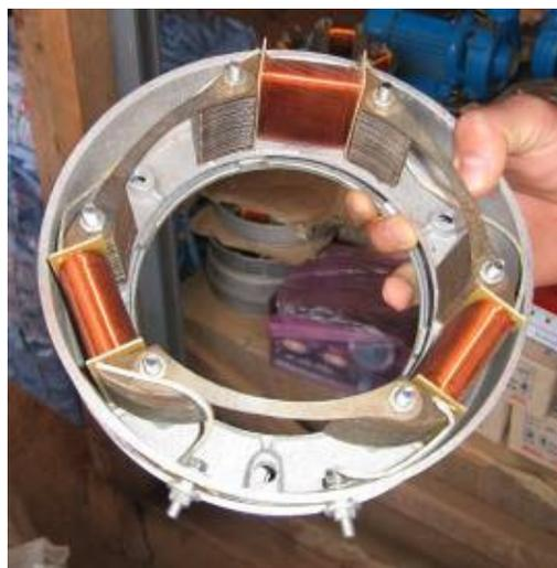
**Figure 27 - New windings for pico-hydro unit**
