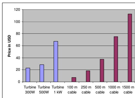
Figure 28 – Average investment costs for different turbines and cable lengths
