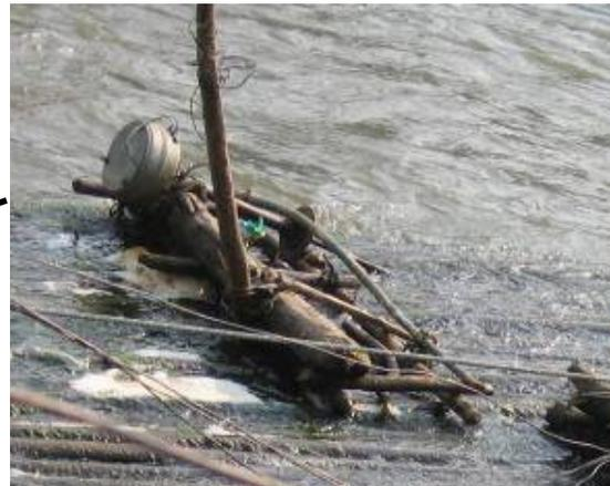
Figure 14 - Pico-hydropower unit on a raft-like structure, near Sop Nhao, Mai district, Phongsali province
