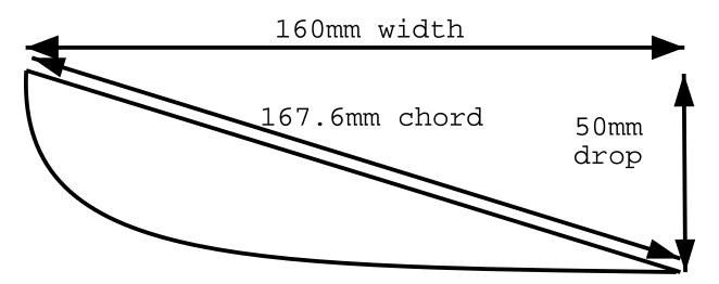
Issue: This is where I got confused. Due to the drop, the width of the cut is not the same as the chord of the airfoil. This is most noticable at the inner sections.
