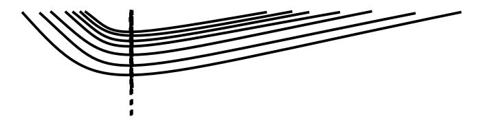
A View of all the sections lined up on the face and the line of the thickest point. This is not the way the blades are constructed, but shows the relative curves of the sections.
