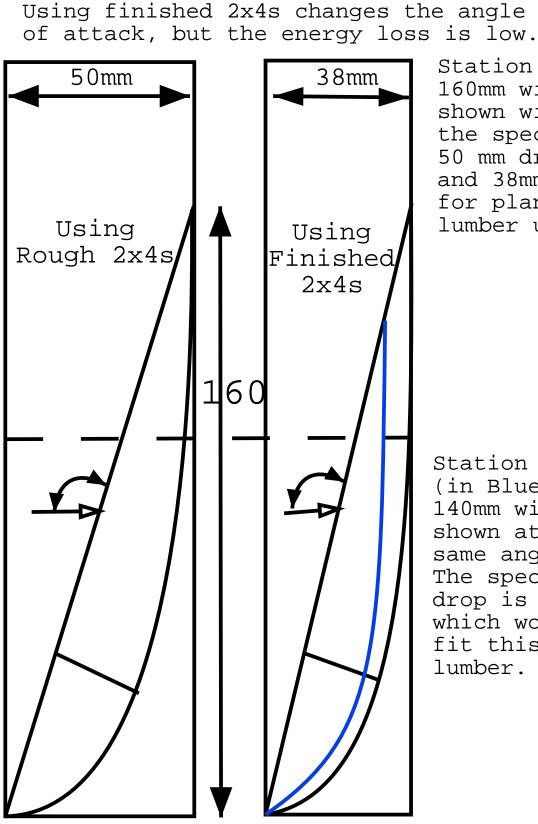
Station 1 160mm width shown with the specified 50 mm drop and 38mm drop for planed lumber use.
