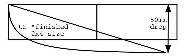
Issue: When using US 2x4 measurements for planed lumber, it is not possible to use the 50mm drop for the first station as recommended in the book since planed 2x4s are actually 1.5"x3.5" or 38mm x 89mm. This is indeed a rip off.
