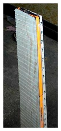
Now grab a hammer and a wood chisel and start making chips... This goes fairly fast but you have to be careful and watch the grain of the wood. You don't want to split into the marked area. On the larger chunks where the cuts went deeper you should take them down a little at a time. I usually start from the tip and work my way down to the root as shown below...
