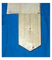
Once the root is cut to a width of 3 ½ inches mark and cut the angles at 120 degrees as shown above from the centerline. This will get them to fit snug in the center for mounting on the prop hub discussed later.
