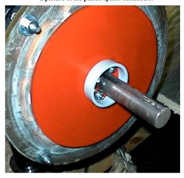
At this point you should bolt the prop assembly together with all nine bolts. They don't have to be torqued at this point but snug them up well. Slide the assembly on the shaft making sure its all the way back against the bolts or spacer and drill a ¼ inch hole through the shaft using the prop mount hub as a guide. Its best to drill ½ way through one side then finish from the other when using a hand drill unless your real good at lining them up.
