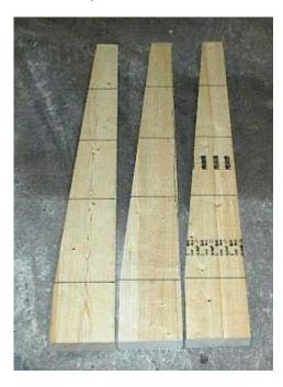
When the un-needed section is cut off then use the square and draw the lines all the way around all 3 blades. Sometimes to make it easier you can number the stations starting from the first line to the root as 1 and the tip being 5. It helps to remove the confusion as we lay out the blade, especially if you've never carved a blade.
