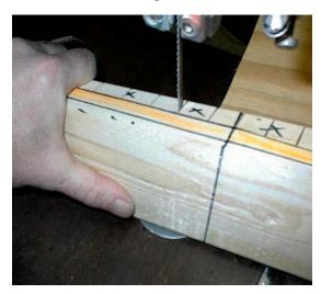
This will cut the slot at the angle you want and leave the leading edge clean with no cuts. Once you're done with all 3 blades you can start on the other side of the blade.
