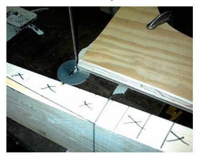
Below shows the board clamped to the band saw...
