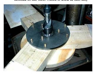
If you don't have a 1 inch drill you can mark the point on the root at ½ inch up toward the tip straight across and this will accomplish the same thing. No more than ½ inch though, it's best to allow the wood to sit on the shaft. You can hone the hole with a larger drill with some sandpaper
