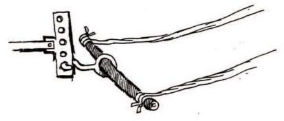
Control of the plough adjustment can be obtained by either increasing or decreasing the rope length between the plough and donkey or by moving the main bar upward or downwards.
