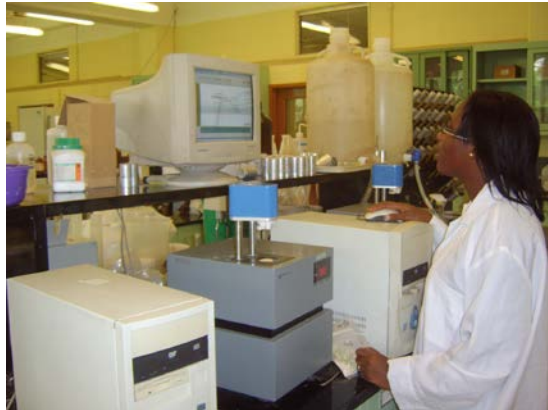
Appendix 11D: Rapid Visco- Analyser being used to determine pasting properties of flour samples
