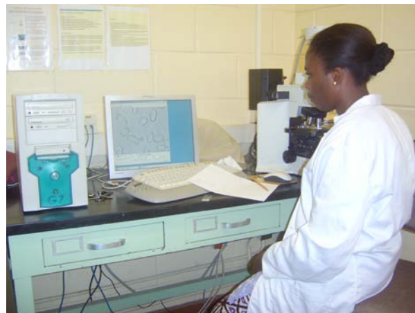
Appendix 11E Compound microscope being used to observe slides of starch granules and take pictures
