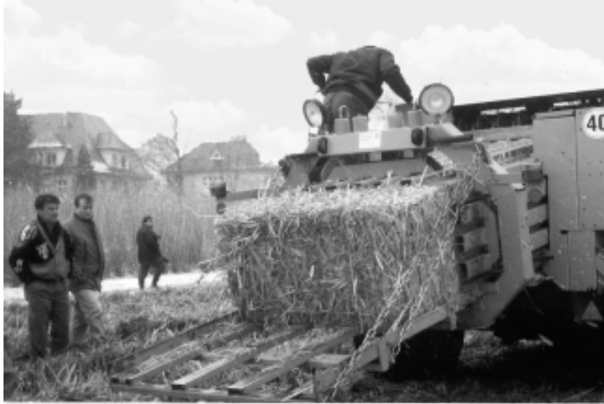
Figure 5. Baling of miscanthus straw from a demonstration plot, using a Claas baler. Photograph taken February 1995, Forchheim, Baden-Württemberg, southern Germany, by Dr. I. Lewandowski, Institute for Crop Production and Grassland Research, University of Hohenheim, Germany. Reproduced by permission. A color version of the image is on the Bioenergy Information Network website photo gallery ( http://www.esd.ornl.gov/bfdp/ ).
