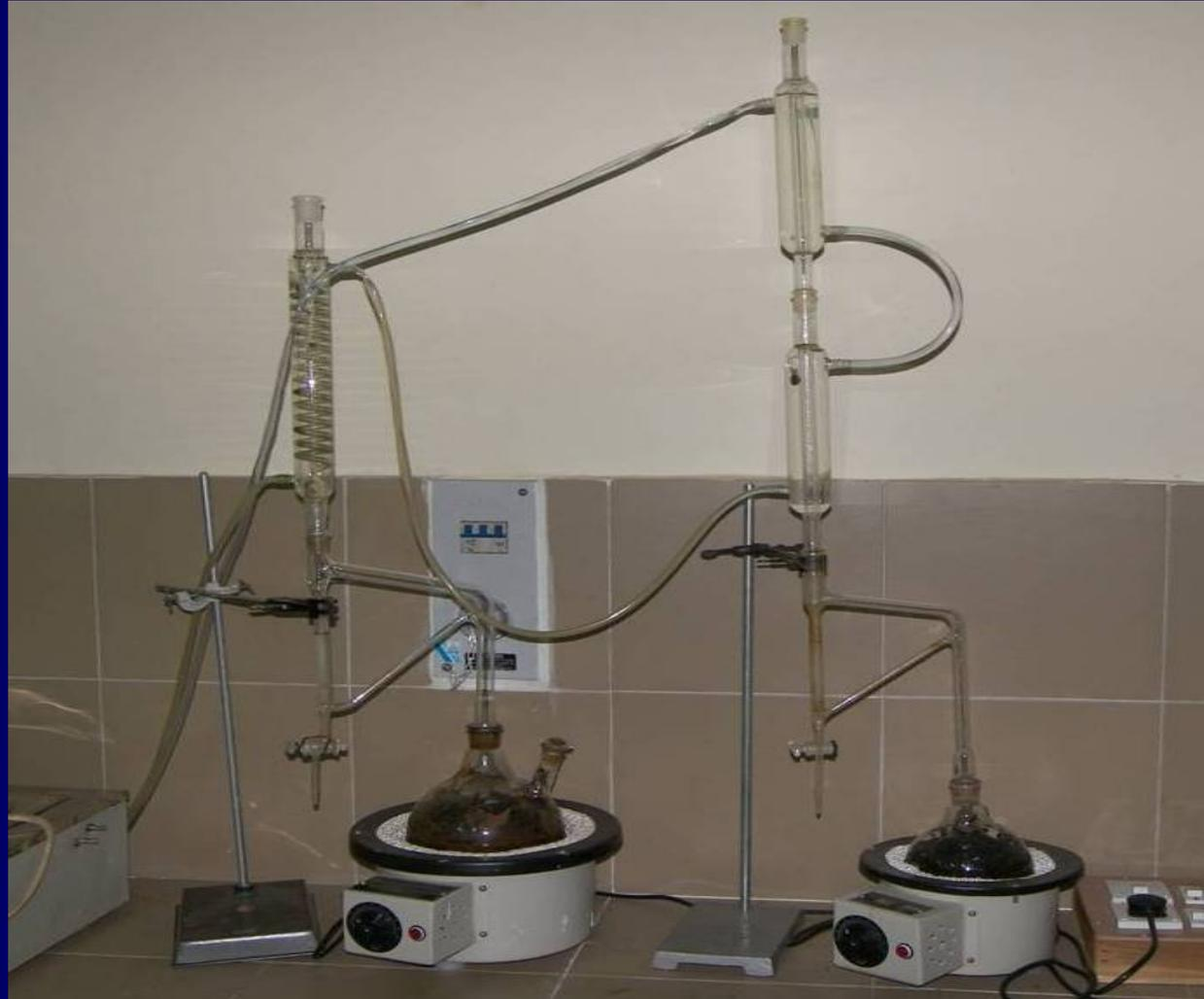
**Extraction of volatile essential oil fractions using Clevenger apparatus**
