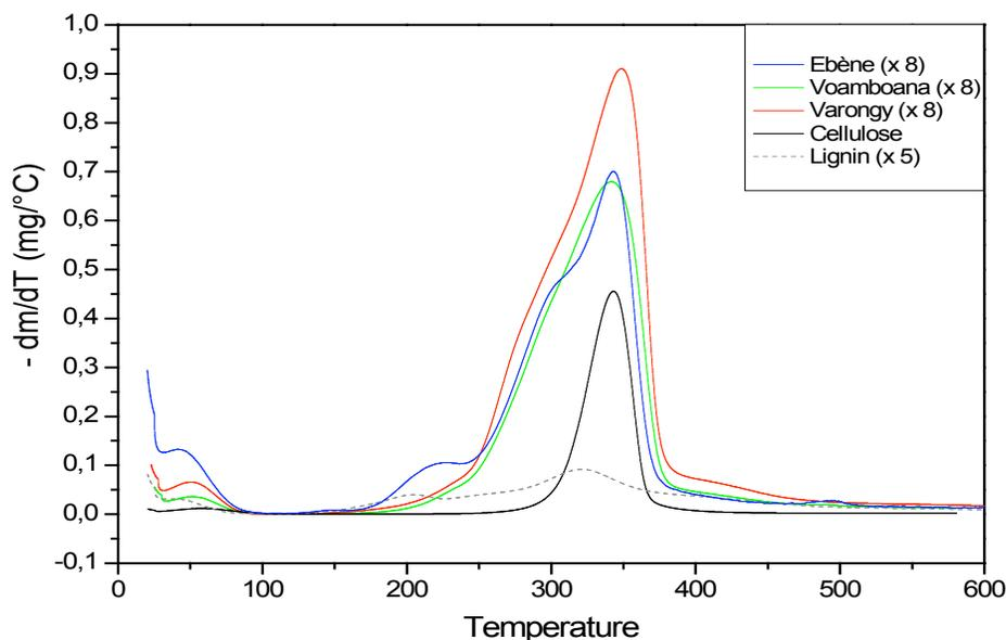
Figure 3: TGD thermograms of the ebony, voamboana, varongy, cellulose, and lignin
