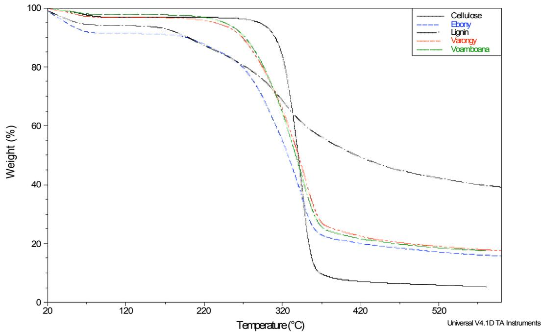
*Figure 2: TG thermograms of three malagasy woods, cellulose, and lignin*
