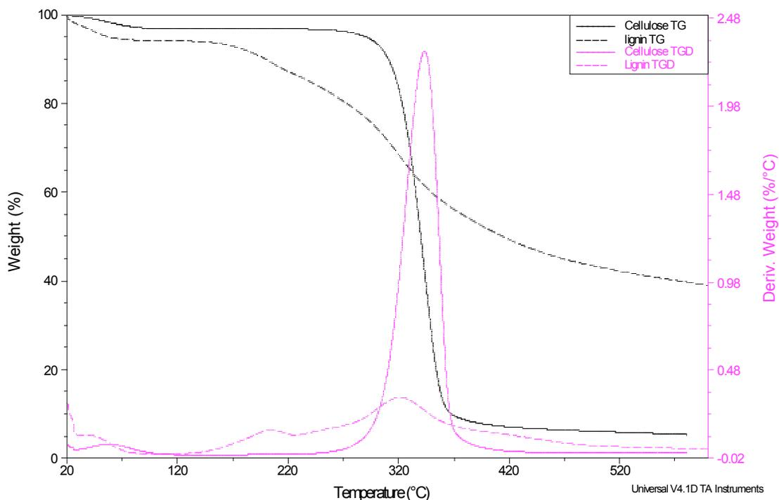
Figure 1: Thermograms (TG and TGD) of cellulose and lignin
