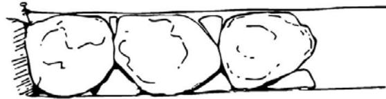
Figure 3: Uneven boulders need to be pinned
