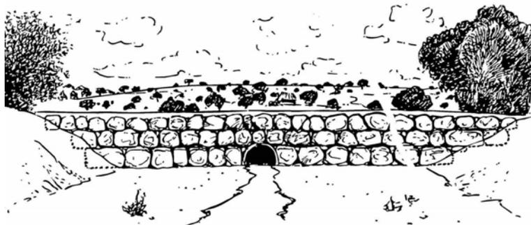
Figure 6: Tying in the ends of the bank
