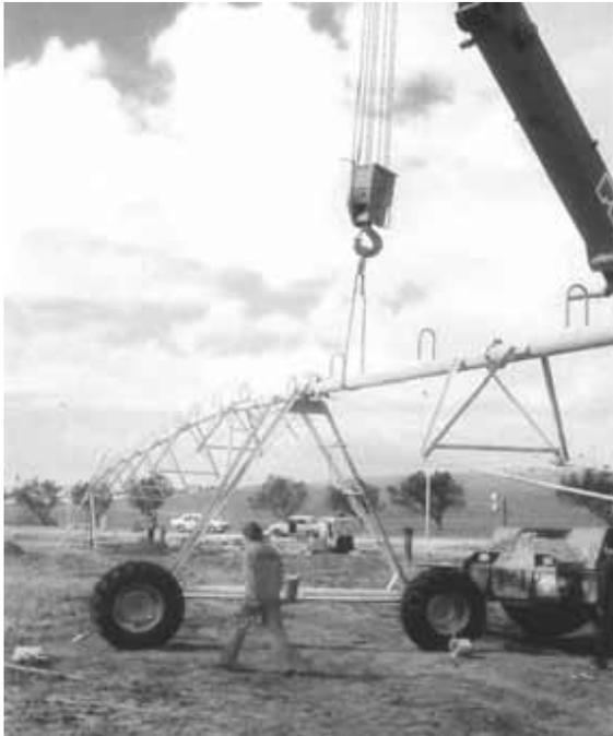
**FIGURE 10.8 - Déplacement du système.**
