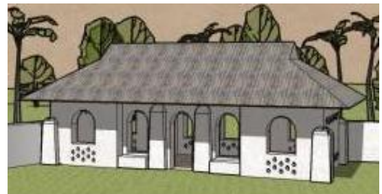
RIGHT: PIERS ALLOW CLOSER WINDOW SPACING
