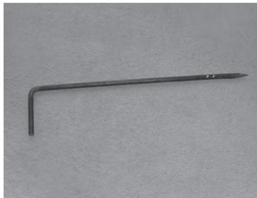
**Figure 4.12** The single bale needle is used for feeding cables, etc. through a bale wall
