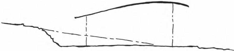
**Figure 2.4** Establish the required cut and fill area
