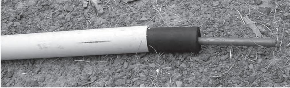
**Figure 13.2** Copper pipe covered with black foam in a PVC pipe
