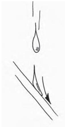
**Figure 9.1** The energy of falling rain is diverted as it strikes a sloping roof
