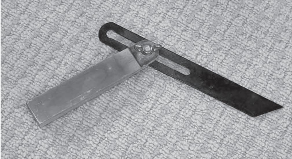
**Figure 8.28** Adjustable bevel
