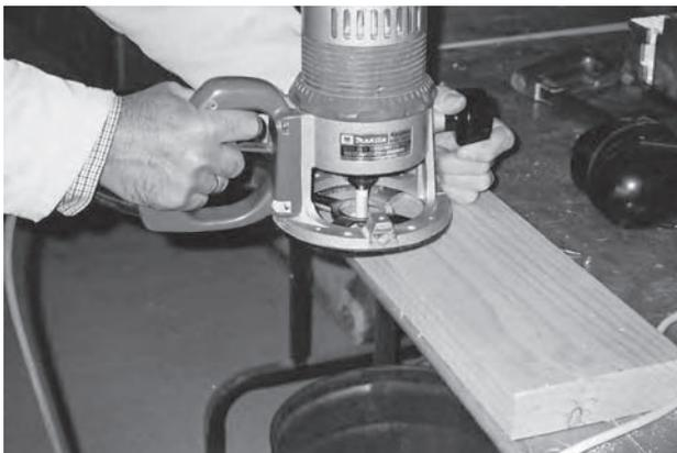
**Figure 14.5** Use a router to remove the bulk of the timber from the hinge checkout
