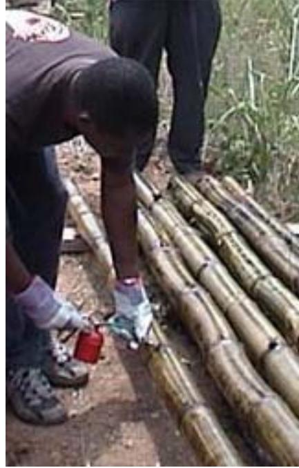
Pictures 1-2: Drilling and Injecting Creosote Oil
