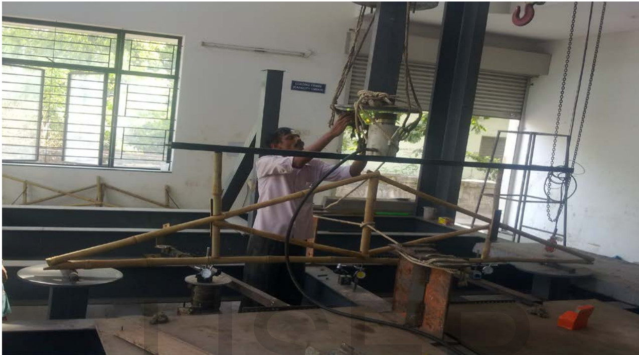
Figure 4.4.A Test set-up for truss testing
