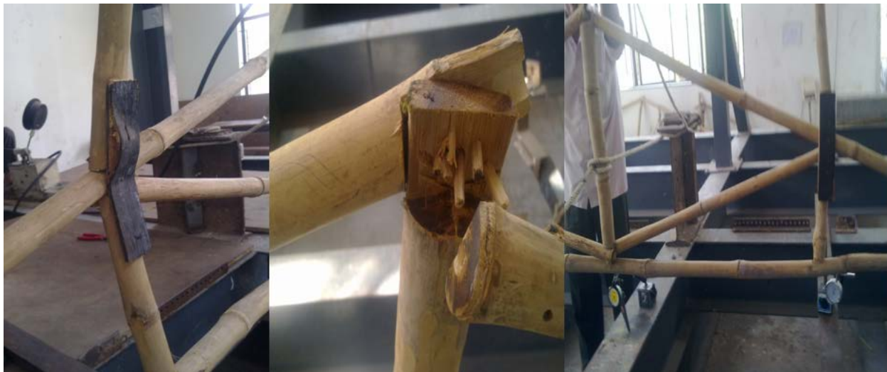
Figure 4.4.B Failure of truss observed during testing
