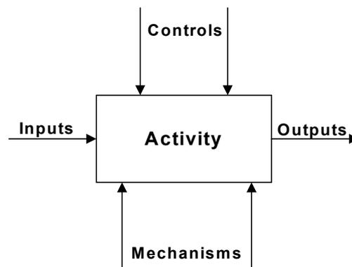
Figure 4.1: IDEFØ Function Box and Interface Arrows (KBSI 2000)
