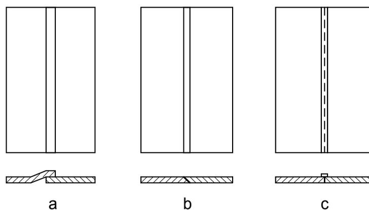
Figure 5.10: **Connection between wall-fillers**
