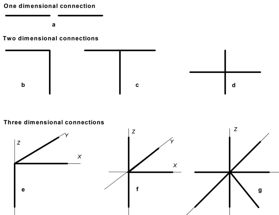
Figure 5.11: **Connection types for a wall**
