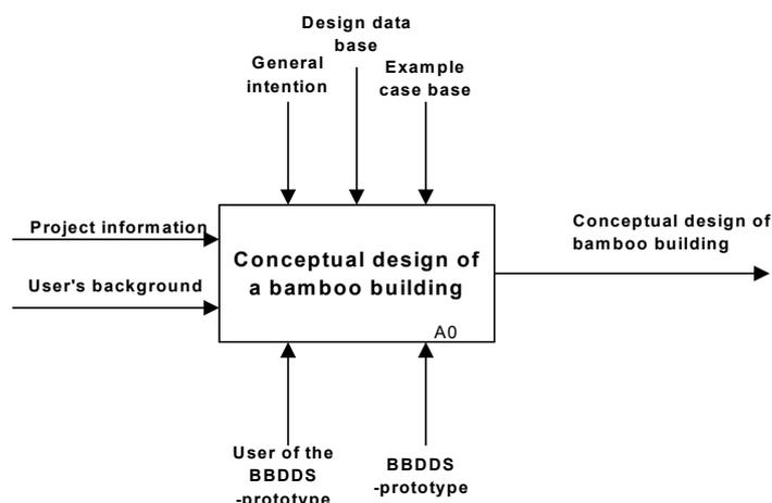
Figure 4.2: Main activity of the conceptual design of a bamboo building
