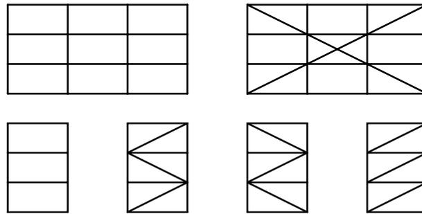
Figure 5.7: Typical frames for a wall structure
