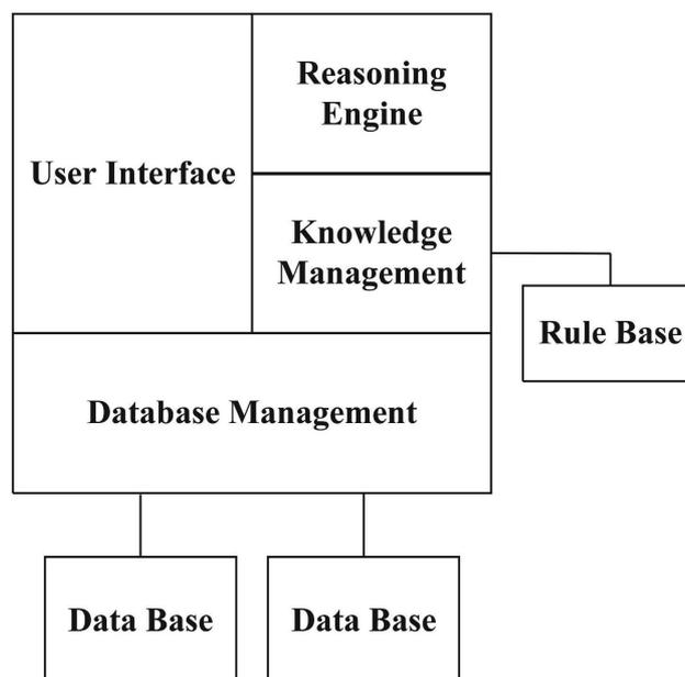
Figure 3.2: **Typical structure of a DSS (after van Zutphen, 1999)**
