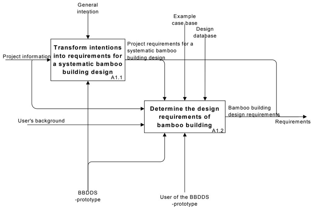
Node: A1 Determine the bamboo building design requirements
