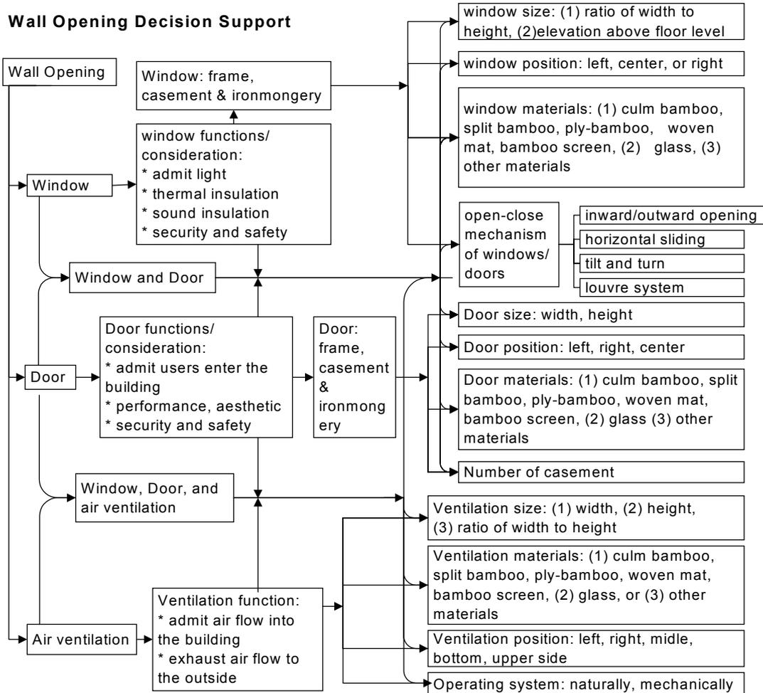
Figure 5.4: Aspects of the design of wall openings (based on Mardjono, et al., 2001, 2002)
