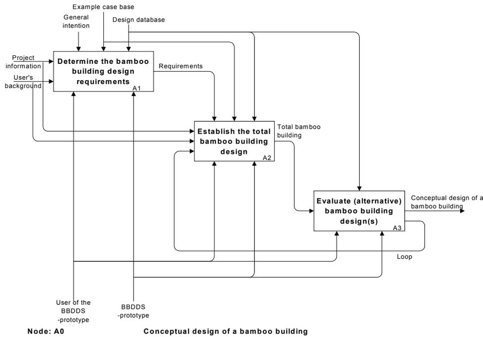
Figure B.2: Decomposition of the conceptual design of a bamboo building
