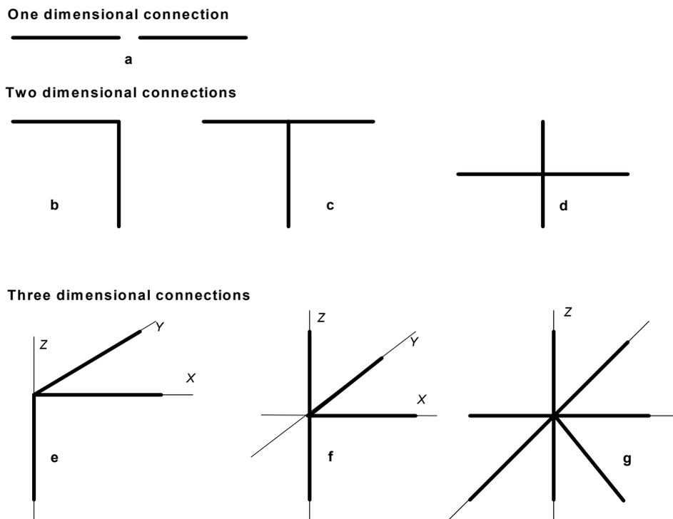
Figure 5.11: **Connection types for a wall**
