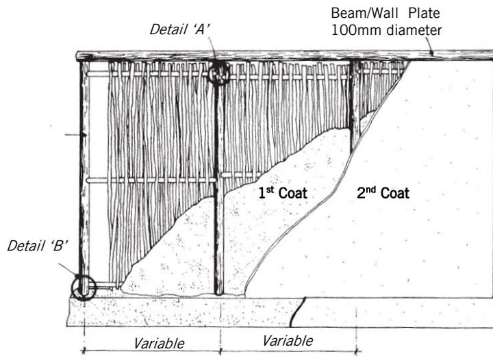
Figure 14: Wall construction Illustration by Duval Zambrano/J. Cuizano
