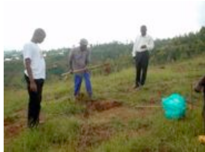
Digging a test pit to analyze soil on site. Uburyo bacukura mu kibanza ngo hapimwe ubwiza bw'ubutaka.
