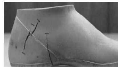
Figure 5. Shows the development of cracks at ankle region
