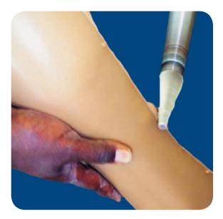
Insert an EVA washer cut to the same shape as the shank about 10 cm below the knee-joint to keep the cosmetic shank in place. This will also prevent creaking.
