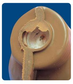
• Grind the distal part until it is flat. Do not remove all the PP.
