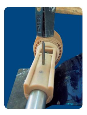
• Remove the excess PP for finishing at the ankle plate.
