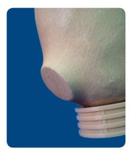
• Cover the mould with a nylon stocking.
