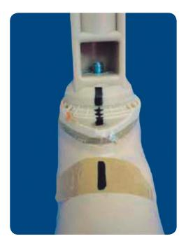
• Remove the foot and draw a line all around the plate 4 mm from the edge.
