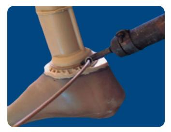
Drill a 5 mm hole in the concave cylinder and the pipe.
