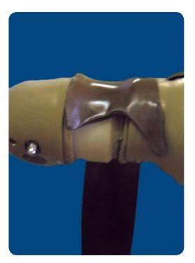
• When the PP has cooled down, grind the edges and weld.
