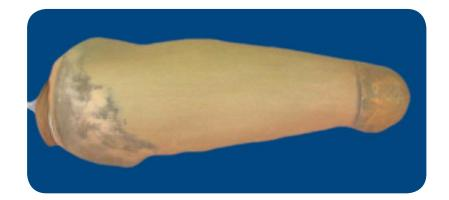
• Drape 4 mm PP around the socket in the same way as for the first socket.
