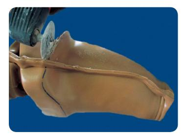
• Grind the distal part of the cup down to the EVA pad.
