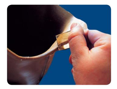
• Using a conical drill, make the hole for the cotton stocking or for the suction valve.
