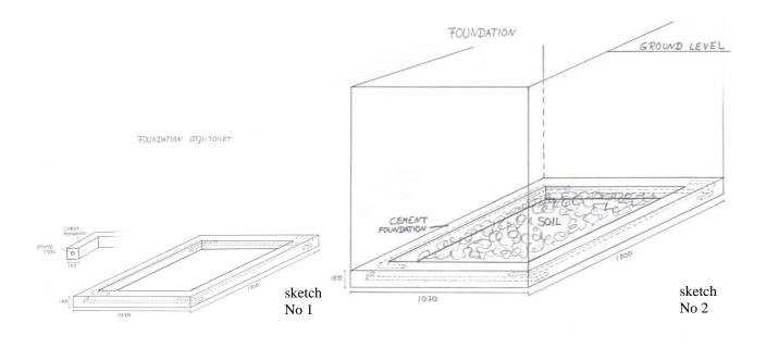
The concrete foundation will be reinforced with the round steel you received together with the Otji-Toilet self builder set. This reinforced foundation has to carry the whole weight of the toilet house and will prevent the walls from cracks. It is important to level the foundation exactly to get a straight toilet house. As a preparation for the concrete foundation dig a square channel of 150 mm depth and 150 mm wide on the ground of the hole.
