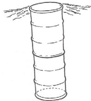
The small volume and the high cost of the drums make this method fairly expensive. If the sides of the drums are not provided with sufficient perforations, absorption of liquids can be a problem. Another problem is that the sheet metal will eventually corrode and collapse if the drums are too old. The pit contents and the resultant gases in a latrine are very corrosive.
