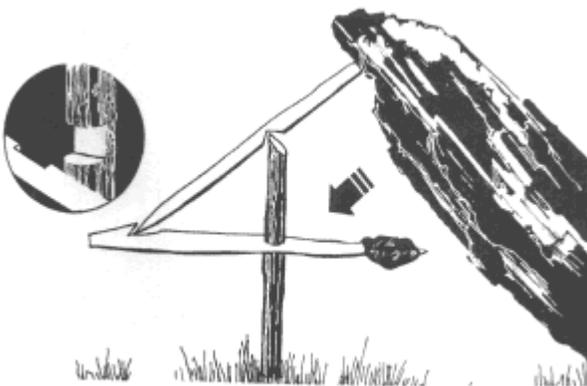
**DEADFALL:** A simple and effective deadfall trap, can be made to any size. A horizontal bait bar is balanced at right angles to an upright with a lock bar, which supports a rock or other heavy weight pivoting around the tip of the upright.
