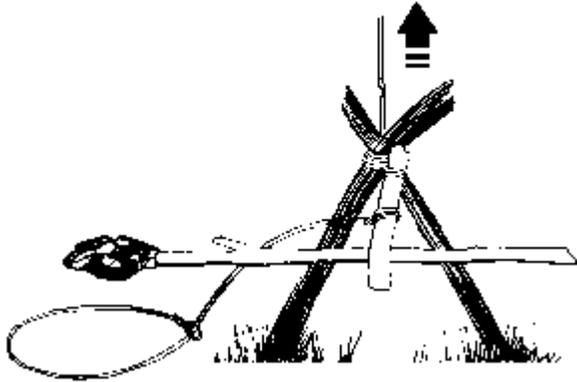
**LEG SNARE:** Push a natural fork or two sticks tied together into the ground. The line from a sapling is tied to a wooden toggle and the toggle passed under the fork. When the game takes the bait attached to a separate stick, it falls away releasing the toggle which flies up taking the snare and the game with it. Large versions are amongst the best snares or heavy game.
