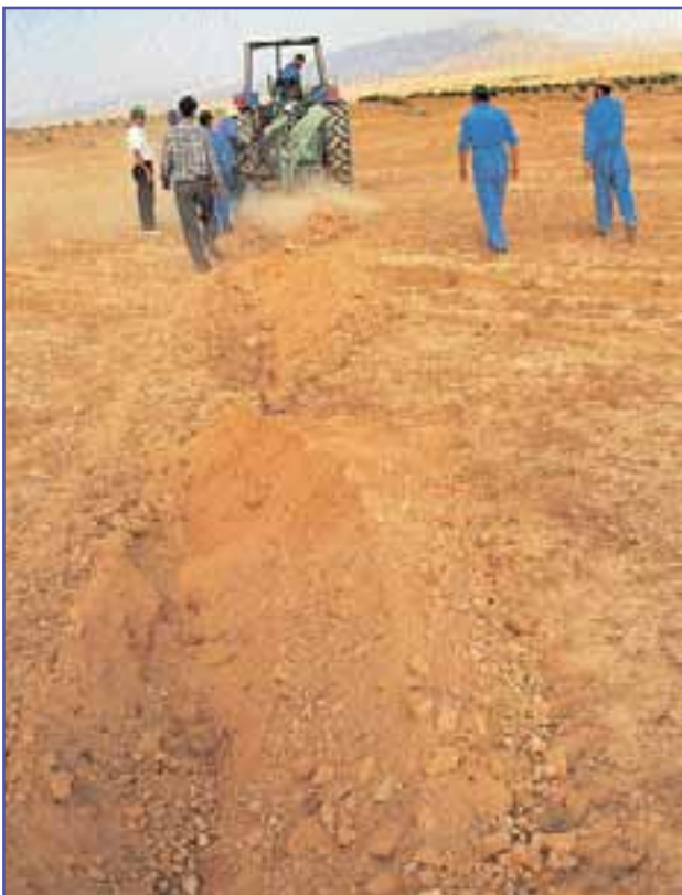
A mechanized implement for making micro-catchments saved labor costs and proved suitable for improving production and reducing degradation in the Syrian badia.
