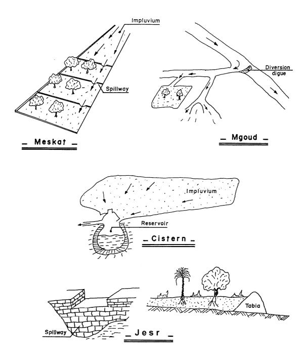
**Fig. 1.** The main water harvesting techniques in Tunisia (adapted from El Amami 1984, Snane *et al.* 1991)
