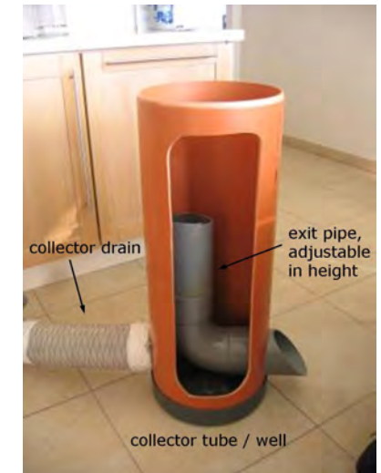
Figure 2. Collector tube well
