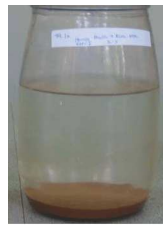
Fig 2. Dirt sink to bottom
