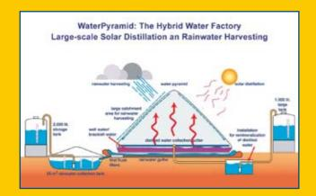
energy needed to clean the water is obtained from the sun. The WaterPyramid is designed following appropriate technology standards, is patented, and rewarded by the World Bank with the Development Marketplace Award 2006 for small scale water innovations.
