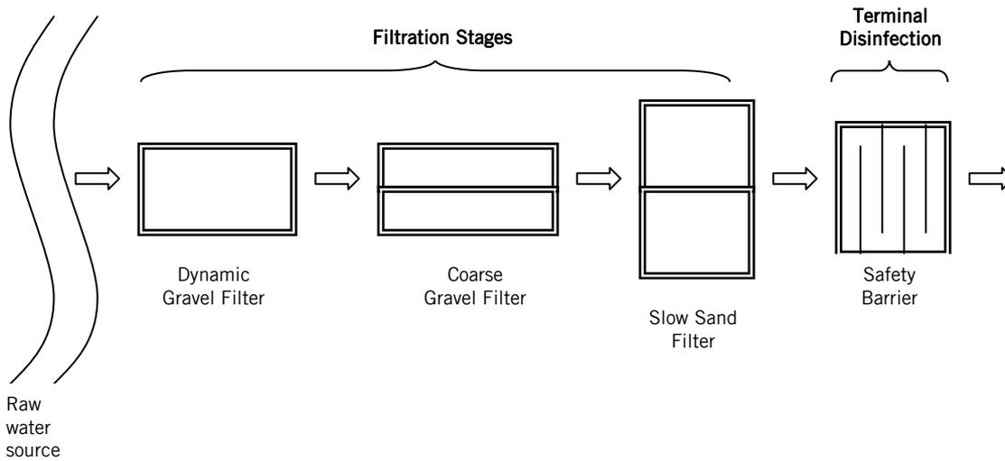
Figure 6: Layout for a multi-stage filtration system (Illustration by A. Elias based on Galvis, G. IRC 2006)
