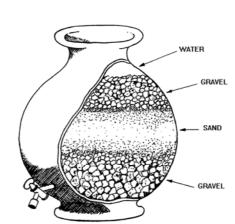
Figure 2: Small-scale sand filter
