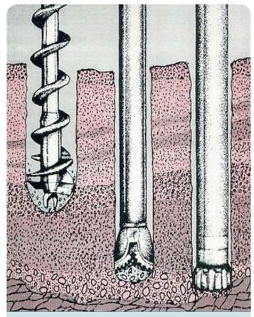
Fig. 2.8 Drill bits for augering, rotary drilling and down-the-<br/>hole hammer© thewaterexperts
