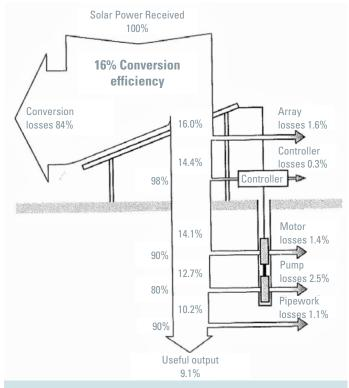
Fig. 3.15 Power flow in a solar pumping system
