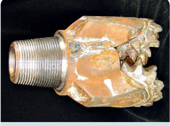
Fig. 2.67 Rock roller bit
