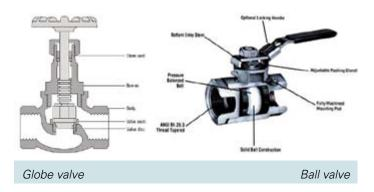
All types and sizes of valves commonly used in piped water supply (for connecting GI, UPVC and HDPE pipes) are detailed below.
