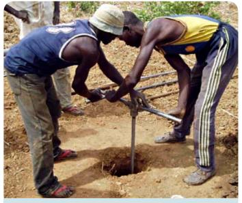
Fig. 2.14. Light hand auger equipment
