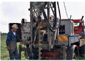
Fig. 2.6 Auger drilling
