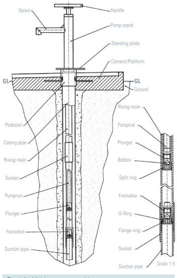
Fig. 1.21 Malda pump assembly
