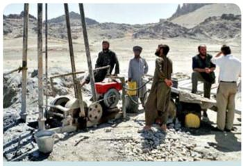
Fig. 2.7 Cable tool drilling, Pakistan
