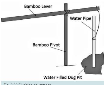
Fig. 2.22 Sludging equipment
