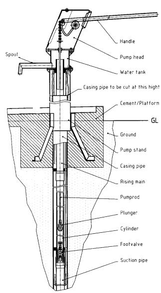
Fig. 1.43 U3M pump assembly
