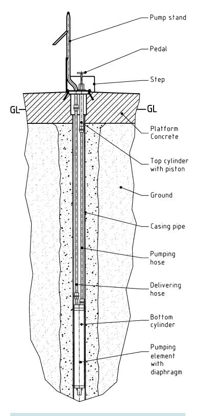
Fig. 1.51 Vergnet Hydropump assembly
