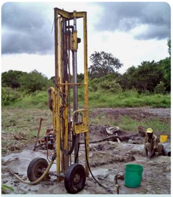
Fig. 2.9 Mud drilling, Tanzania
