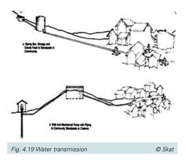
household taps through a distributution network consisting of pipes and fittings laid in trenches. The distribution network can also include various types of control valves, pressure release devices, water meters and other fittings.
