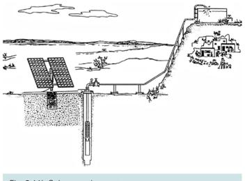
Fig. 3.11b Solar pumping system
