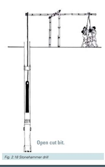
percussion drilling. If temporary casing is used, considerable time and suitable tools are needed to drive it into the ground and remove it. Depths of 20 to 30 m are possible if there is no temporary casing required, otherwise the limit is about 15 m.
