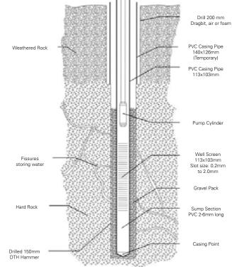
Fig. 2.59 Typical design drawing of lined borehole in consolidated formation with risk of collapse
