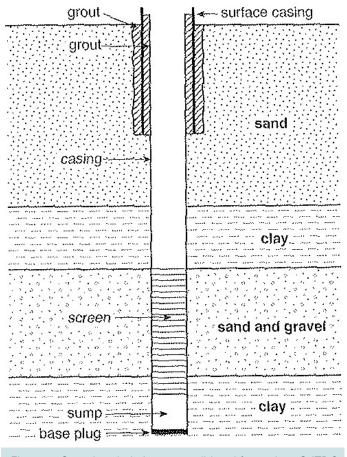
Fig. 2.36 Open borehole in unconsolidated formation © ITDG
