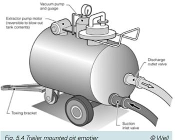
Fig. 5.4 Trailer mounted pit emptier
