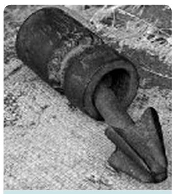
Fig. 2.25 Drill bit with footvalve above
