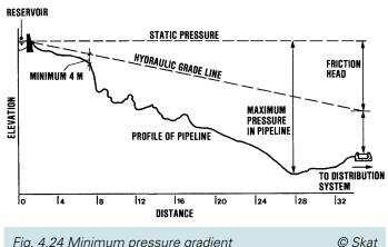
Fig. 4.24 Minimum pressure gradient
