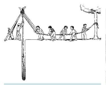
Fig. 2.17. Schematic of hand percussion rig
