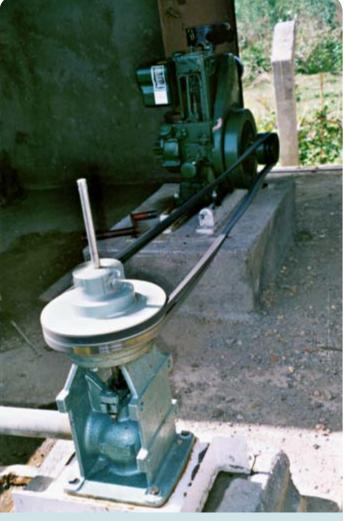
Fig. 4.16 Progressive cavity pump, Eritrea
