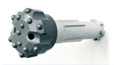
Fig. 2.68 Down-the-hole hammer
