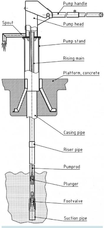
Fig. 1.4 Lever action pump
