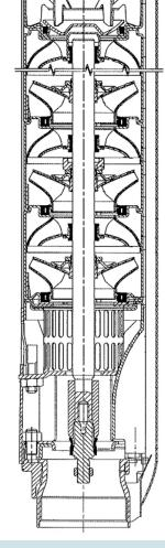
Fig. 3.13 Centrifugal pump
