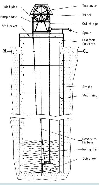
Fig. 1.16 Nicaragua rope pump assembly
