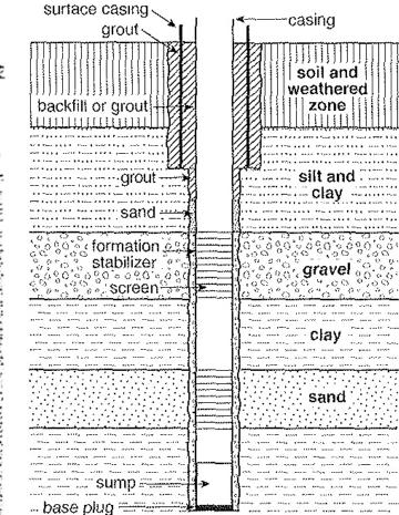
Fig. 2.35 Cased borehole in unconsolidated formation © ITDG
