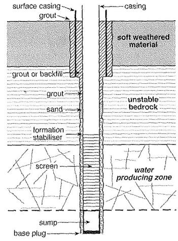
Fig. 2.39 Cased borehole in consolidated formationwith risk of collapse© ITDG
