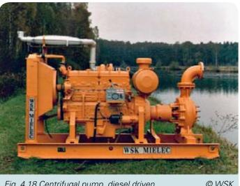
Fig. 4.18 Centrifugal pump, diesel driven
