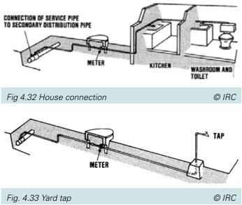
pressure piping (at considerable cost savings). Pipes for distribution systems with house connections generally have to be of a higher pressure class.
