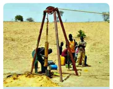
Fig. 2.16 Hand percussion rig in action
