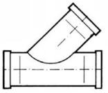
L) Tee 45°, equal female threads, galvanized
