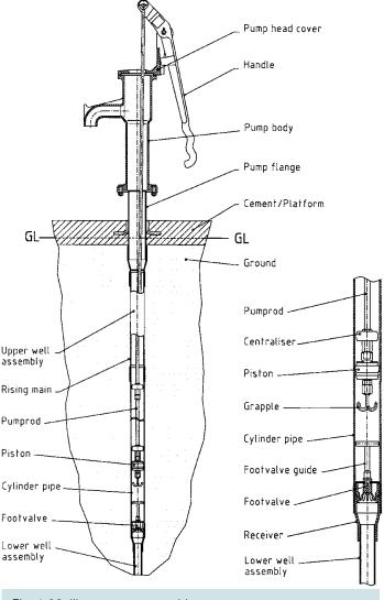
Fig. 1.26 Jibon pump assembly
