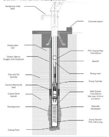
Borehole in unconsolidated material, naturally developed - Lined with 4" (113 x 103 mm) PVC Casing and Screen
