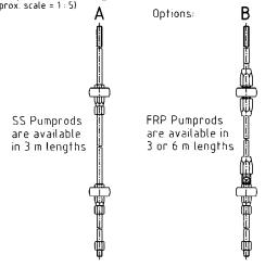
Fig. 1.44c Options for the U3M pump
