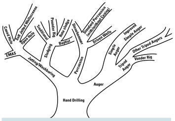
Fig. 2.12 Hand drilling family tree
