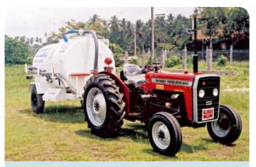
Fig. 5.7 The Sri Lankan tractor-drawn trailer-mounted vacuum tanker © UNICEF Sri Lanka
