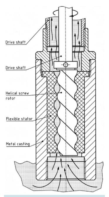
Fig. 1.7 Progressive cavity pump
