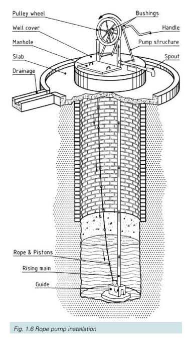
The rope pump is not defined by a specific design but by a concept. Worldwide many different rope pump designs, adapted to their local conditions, are produced locally in small workshops near to the users. The producers need to study the potential market and economic viability carefully. Areas with a high density of dug wells usually have a big potential for rope pumps.
