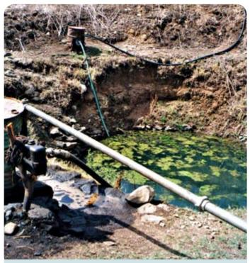
Fig. 3.16 Spillage from a diesel pump
