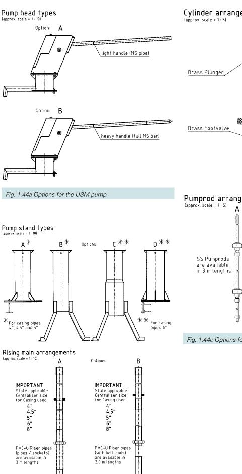
Fig. 1.44b Options for the U3M pump
