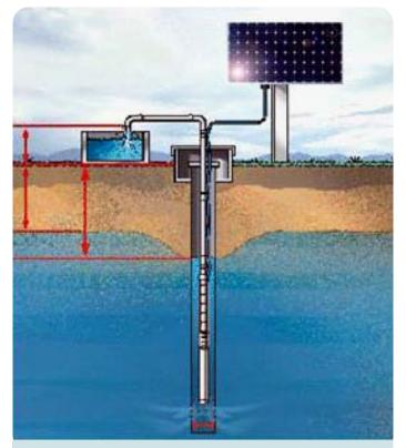
Fig. 3.11a Solar pumping system
