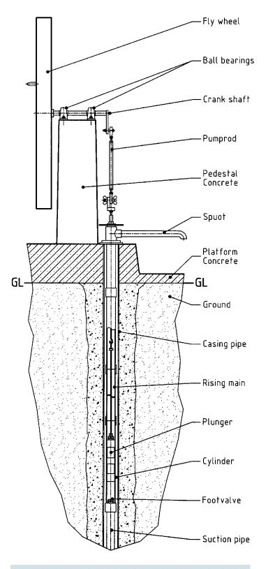
Fig. 1.49 Volanta pump assembly
