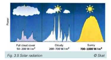
radiation consists of about 40% direct radiation and 60% diffuse radiation. Both direct and diffuse radiation are converted into electricity by solar cells.
