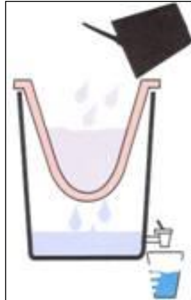
Cross Section of Ceramic Pot Filter (Credit: Filter Pure Inc)
