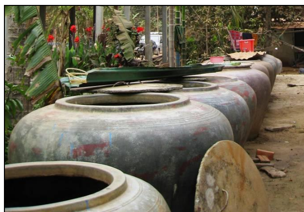
Passive Oxidation in locally available water jars (Credit: T. Ngai)
