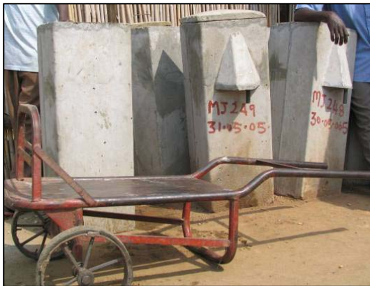
Transporting filters with a specially constructed dolly
