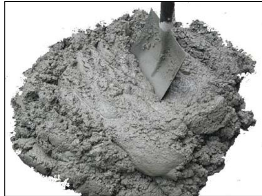
The consistency of the concrete should be fairly stiff and dry. The filter is prone to cracks or leaks if too much water is added.
