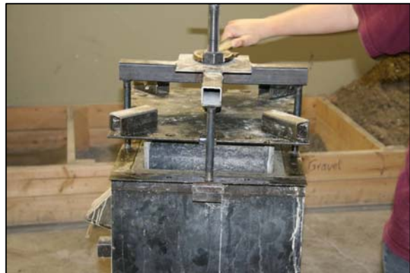
Step 8 – Tightening the nut on the extractor to remove the interior mold
