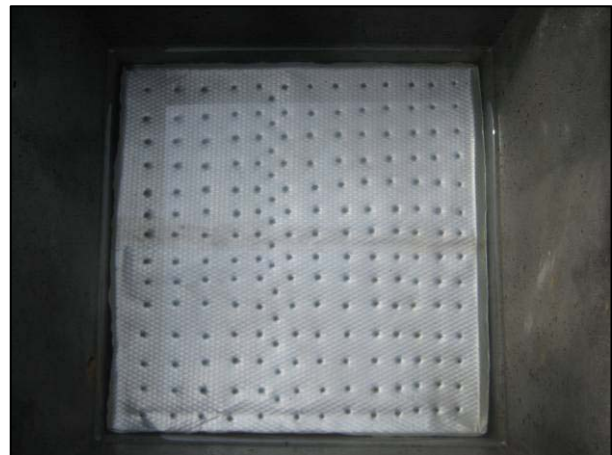
This is an example of a bad diffuser. It has too many holes - only 100 holes are needed.
