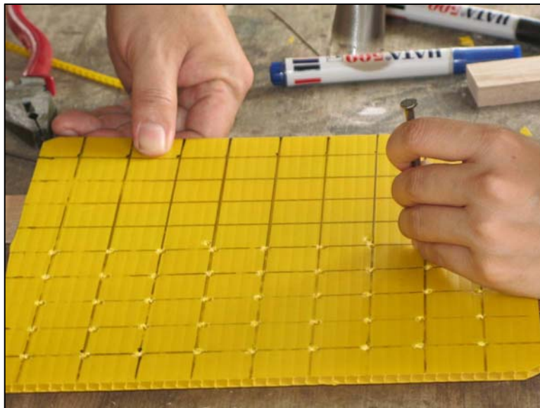
A corrugated plastic diffuser with well placed holes
