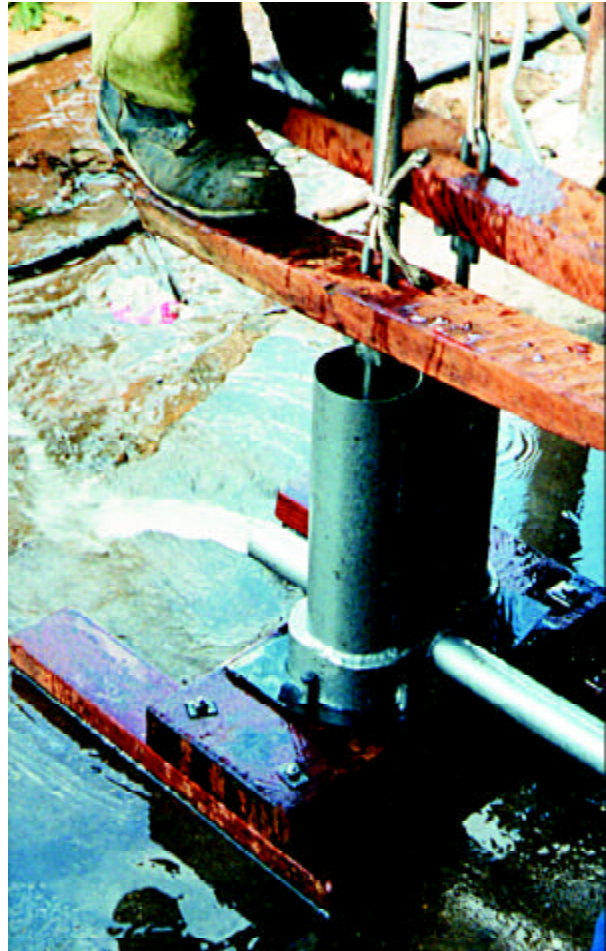
Figure 8: Masvingo treadle pump (pressure delivery), under test at manufacturers
