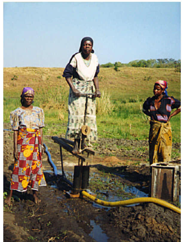
Figure 16: Treadle pump (pressure delivery), Malawi. Suction pipe is yellow corrugated plastic; delivery is through blue lay-flat hose
