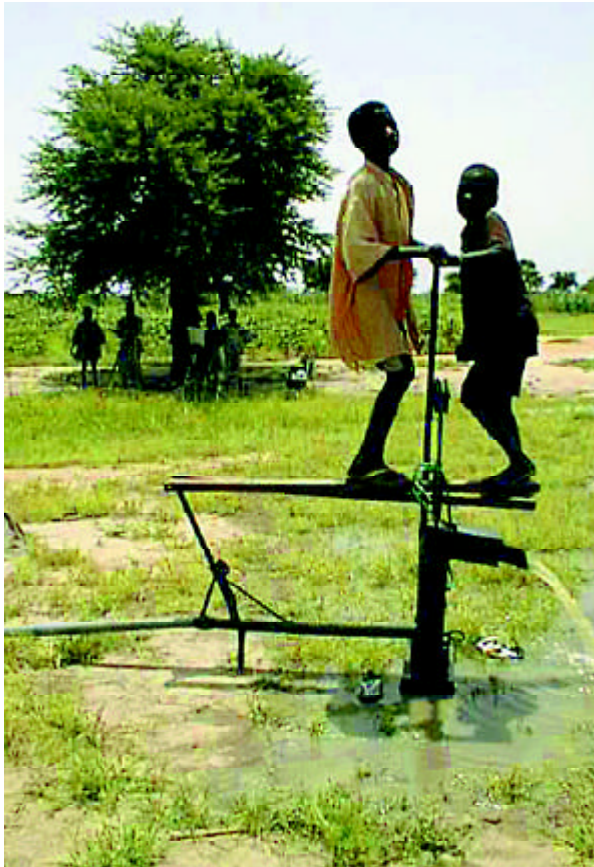
Figure 9: Bielenberg pump, Niger
