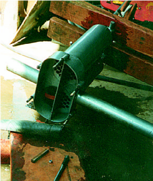
Figure 7: Masvingo treadle pump (pressure delivery), close-up of under-side
