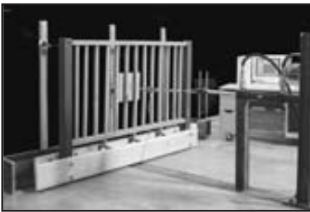
Testing a railing at the WMEL.
