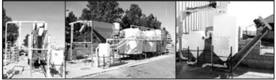
Washington State University Pilot-Scale Manure Digester
