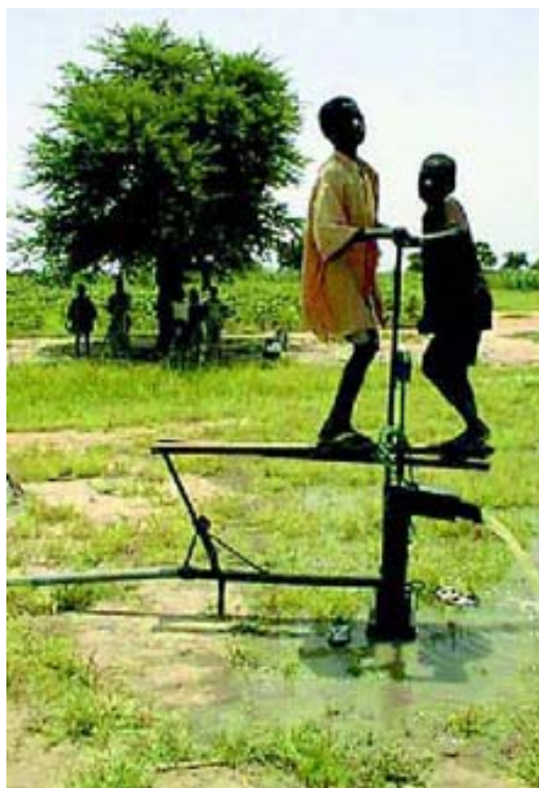
Figure 9: Bielenberg pump, Niger
