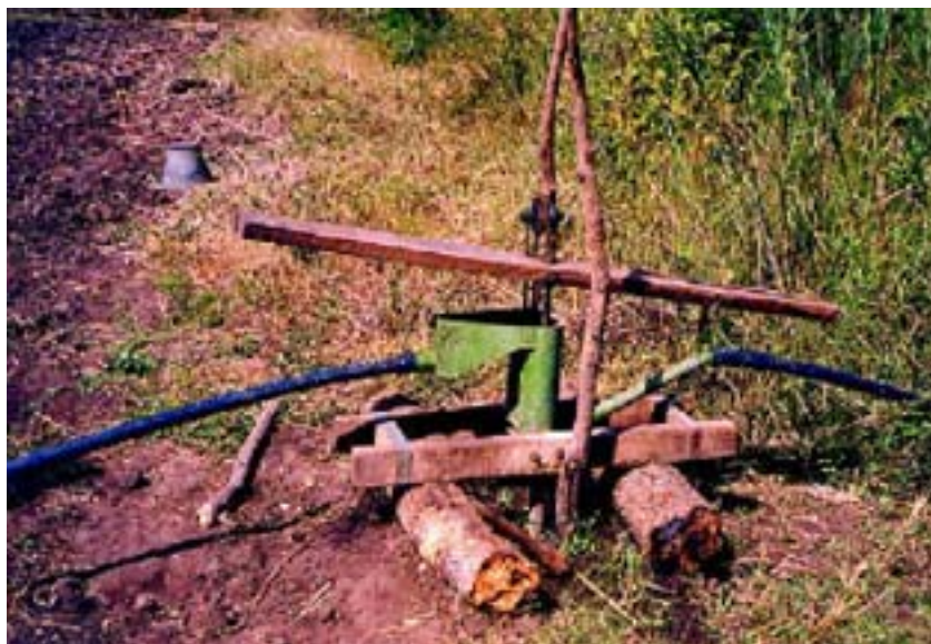
Figure 5: IDE modified river pump, Zambia
