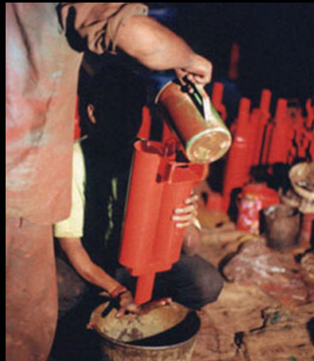
Photo: Testing for leaks
