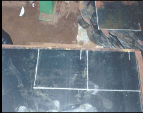
1. Metal components are cut from sheet steel
