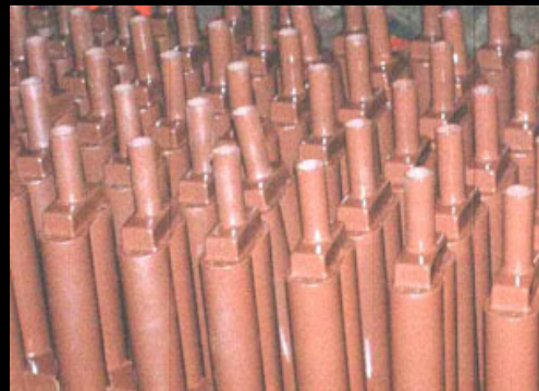
5. The cylinder and plunger sub-assemblies are painted and the cylinders tested for leaks
