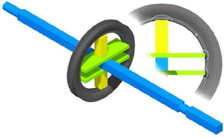
**9.** Attach the handle to the axle with two planks of wood. The optimal distance between the handle and the axis is approximately 20 cm. The end of the handle is rounded, so that a piece of the PVC pipe fits the handle and can move freely.
