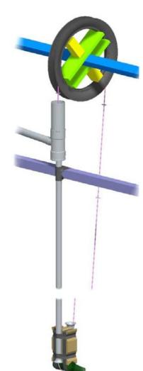
**25.** Assemble the PVC T-joint with the discharge pipe and the wider pipe as shown in the picture below.
