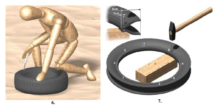
8. Complete the wheel by assembling two planks and two short balks on the axle within the half tires. These planks and balks must be just slightly greater than the inside diameter of the tire (indicated by the circles). The tire than traps the components together on the axle. Nails or screws can be applied but are not necessary. The planks and balks should not be too large since the wheel will become square in that case.
