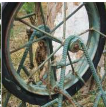
Upper part of a pump installed by Viltec
