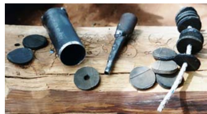
Rubber pistons made of car tire
