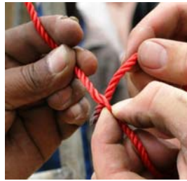
1. making a loop by threading the rope back
