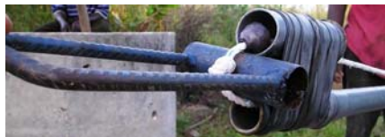
guide box with rope and pistons running through.
