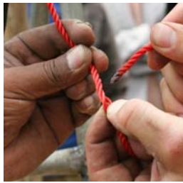
1. making a loop by threading the rope back
