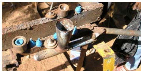
PE piston mould and extruder
