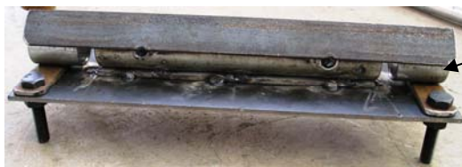
welding jig, bushings
