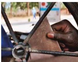
measuring angle with an equilateral triangle
