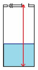
2. Measure the distance from the bottom of the guide box to the end of the PVC pipe (1) and from the bottom to the inlet of the guide box (2)
