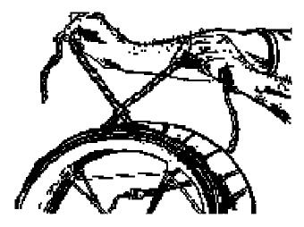
5) Take the two ends and braid them together as shown above, then put the rope back on the pulley wheel. The tension is correct when the rope does not slip or slide back over the pulley wheel while pumping water.
