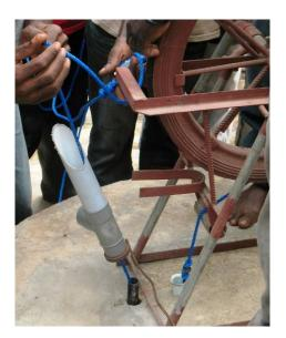
2) Fix the T pipe to the PVC pipe. Centralise the T pipe according to the position of the metal frame and the wheel
