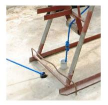
1) Place the front of the wheel basement between the two holes of the cover, centralize it
