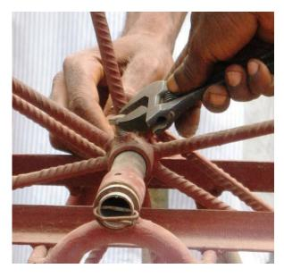
3) Use the spanner to tight the bolts of the axle
