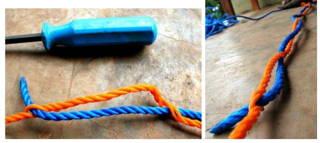
8) Once you have finished this process, seam the extremity. Help yourself using thin biding wire firmly tied
