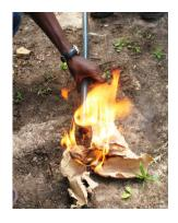
2) The flare is made by heating the end of the pipe and then opening it up with a small PCV pipe of the same diameter. Push this flare tool (small pipe) into the hot end pipe before it cools down. Keep it inside the flare until it goes cool.
