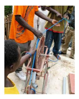
Place the rope, with the desired tension, over the pulley wheel to indicate where the knot should be made. Remove the rope from the pulley wheel and cut it, leaving about 40 extra centimetres at each end. Burn the ends with a cigarette lighter or matches and twist them while they are hot
