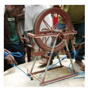
2) Thread a pin to fix the handle. Use the pliers to bend it
