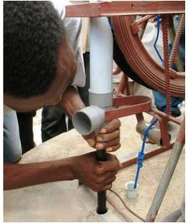
3) Fix the T-pipe to the frame with biding wire.
