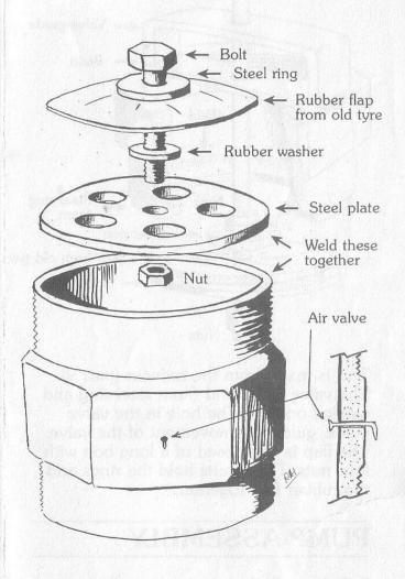
The one way valve is constructed from the 3" double nipple (part 4). One end of it is welded with a 6mm steel plate. Several holes are then drilled in the plate. The center hole is to hold the rubber flap, and the others are water ways.
