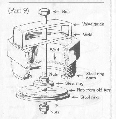
This is made from the reducer (part 9). The valve guide and 6mm steel ring and welded on to it. The hole in the valve guide, guide the movement of the valve. The flap is composed of a long bolt with four nuts. These nuts hold the rings and the rubber flap together.
