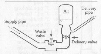
When the check valve is pushed down to start the pump, the water rushes down the supply pipe. In the process, the water sucks the valve up, closing it with a thud. The inertia of water still flowing in the supply pipe, charges the air chamber. The increased pressure, drives some water up the supply pipe, and when the rush of water stops, there is a small bounce back. This bounce back, causes a momentary drop of the pressure, causing the valve to drop open, and the process is repeated again.
