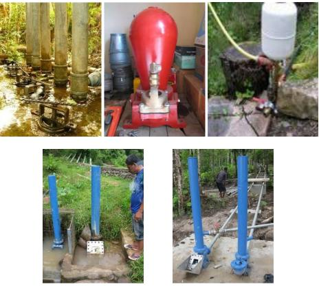
Figure 10: Example of Hydraulic Ram Pumps around the world
