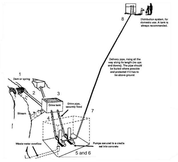
Figure 4: Hydraulic Ram Pump System
