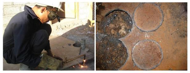
Figure 28: Cutting the iron plate
