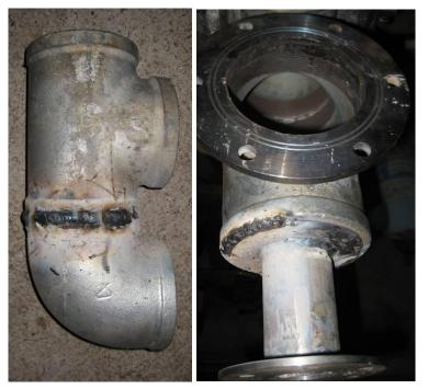
Figure 30: Welding the pump body
