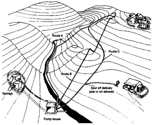
Figure 24: Choice of route for the delivery pipe
