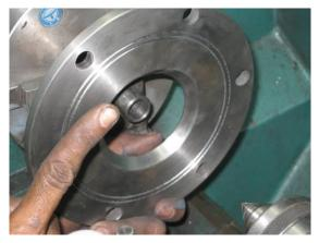
Figure 36: Manufacture of the bottom of the impulse valve plate
