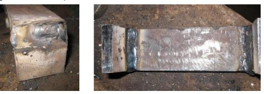
Figure 34: Manufacture of the support for the impulse valve guide
