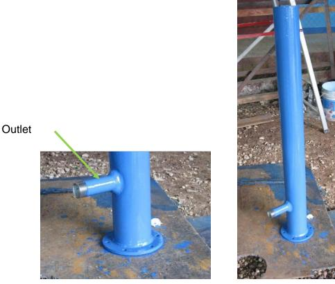
Figure 15: Air vessel
