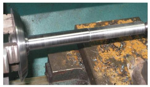
Figure 37: Manufacture of the stem of the impulse valve
