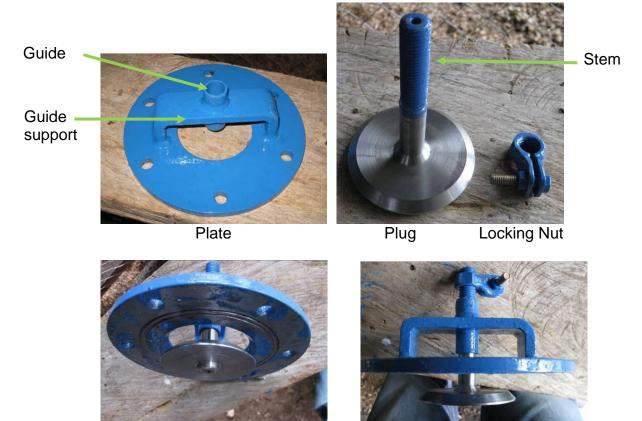
Figure 13: Impulse valve and its components
