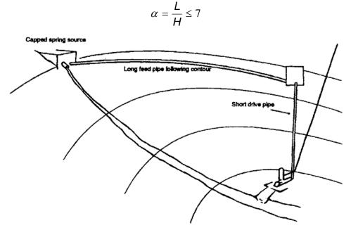
Figure 18: Topography and drive pipe position
