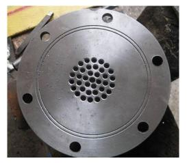
Figure 33: Delivery valve manufacture
