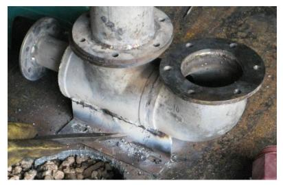
Figure 12.b: Pump body with supports, flanges and reducer
