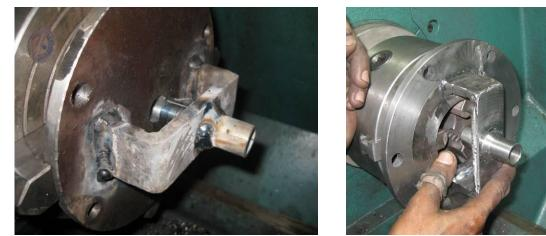
Figure 35: Manufacture of the top of the impulse valve plate On a second time, the bottom side of the stop bar faces the cutting tools:
