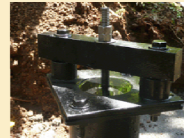
Drive Pipe - supplies the ram pump with water for a proper operation
