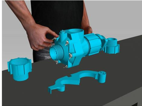
Tighten the Wing Nuts (15) using the 'C' spanner (16), turning 90° only
