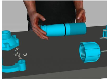
Re-assemble the Shaft (3) and the Adjuster (4) using the 'C' spanner (16).
