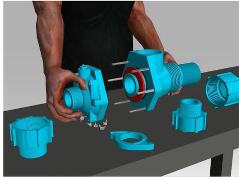
Remove the Main Seal (11) using the 'C' spanner.
