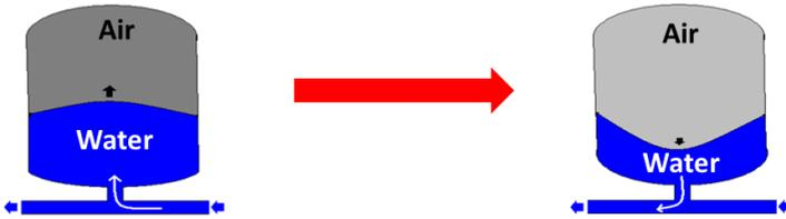
When pulse water enters the accumulator from the pump, the diaphragm is pushed upwards and air in the chamber is compressed to a high pressure.
