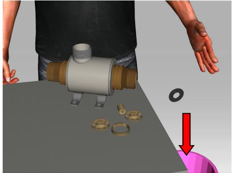
Refit one Valve Seat (13) followed by the new NRV Valve member (8), the Valve Spigot (12), the second Valve Seat (13) and finally the Valve Spacer (14)
