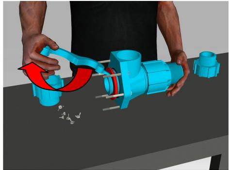
Clean the mating faces of the Body (1) and the Cone (2) and reassemble.
