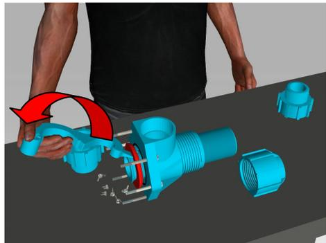
Remove the 'o' ring (14) then extract the Shaft (3). Discard the seal (11) and the 'o' rings (12) & (14).
