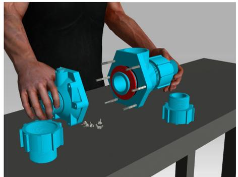
Re-assemble the Wing Nuts (15) by hand.
