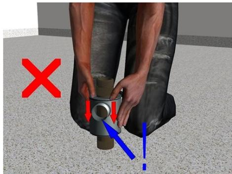
The Main Valve member (9) will be left inside the Main Body (1). Extract it and dispose, then clean all the parts ready for re-assembly
