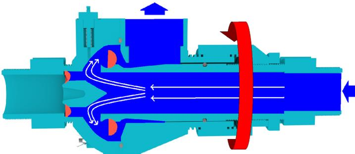
Turning the adjuster to open the valve allows flow through the pump to be regulated so that a greater flow generates a greater pressure and water delivery.
