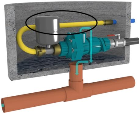
**Set air pressure to equivalent delivery head pressure before attaching pressure vessel.**
