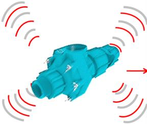
Pump Shakes excessively during operation
