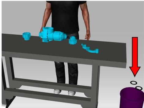
Unscrew the Lock Nut (5) and then remove the Adjuster (4) and all the Wing Nuts (15) using the 'C' spanner (16).
