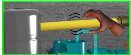
Adjust air pressure in accumulator so that pulse in pipe is at a minimum
