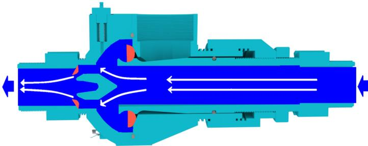
As the flow increases around the main valve a differential pressure occurs causing the valve to suddenly close. The flow and mass of water is then directed through the non-return valve and into the delivery port at a higher pulsed pressure. This pressure suddenly reduces causing the main valve to reopen and the cycle to repeat.
