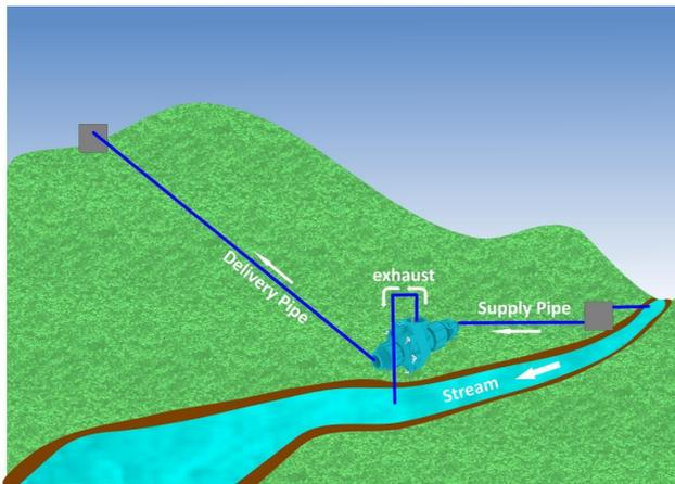
By utilising a naturally flowing water source the Papa pump is able to transport up to 30% of that water to the desired location, allowing the residual water to be returned to the natural source. With minimal maintenance and zero fuel costs and emissions, the Papa Pump will provide you with a clean and efficient solution to your water transportation requirements including agriculture, horticulture, irrigation, domestic and industrial use.
