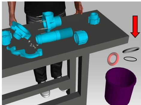
Taking the Cone (2), remove the 3 One-way Valves (8), noting orientation. Discard and replace the worn One-way Valve components (8).
