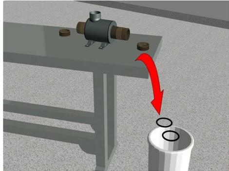
Holding the delivery end of the Barrel (2), pull it from the Outer Casing (1) in the direction of output, taking care not to damage the threads
