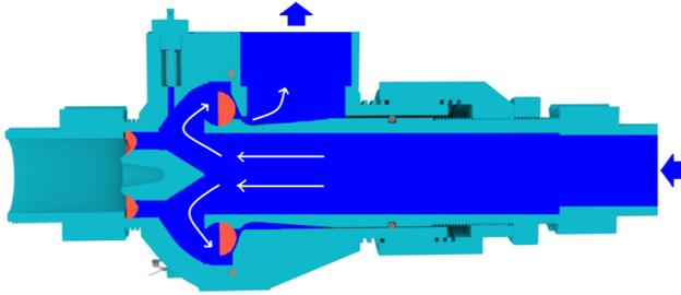
Water enters pump via supply port and flows around main valve to exhaust port.
