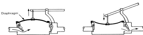
Figure 8: Diaphragm pump
