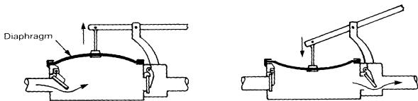
Figure 8: Diaphragm pump
