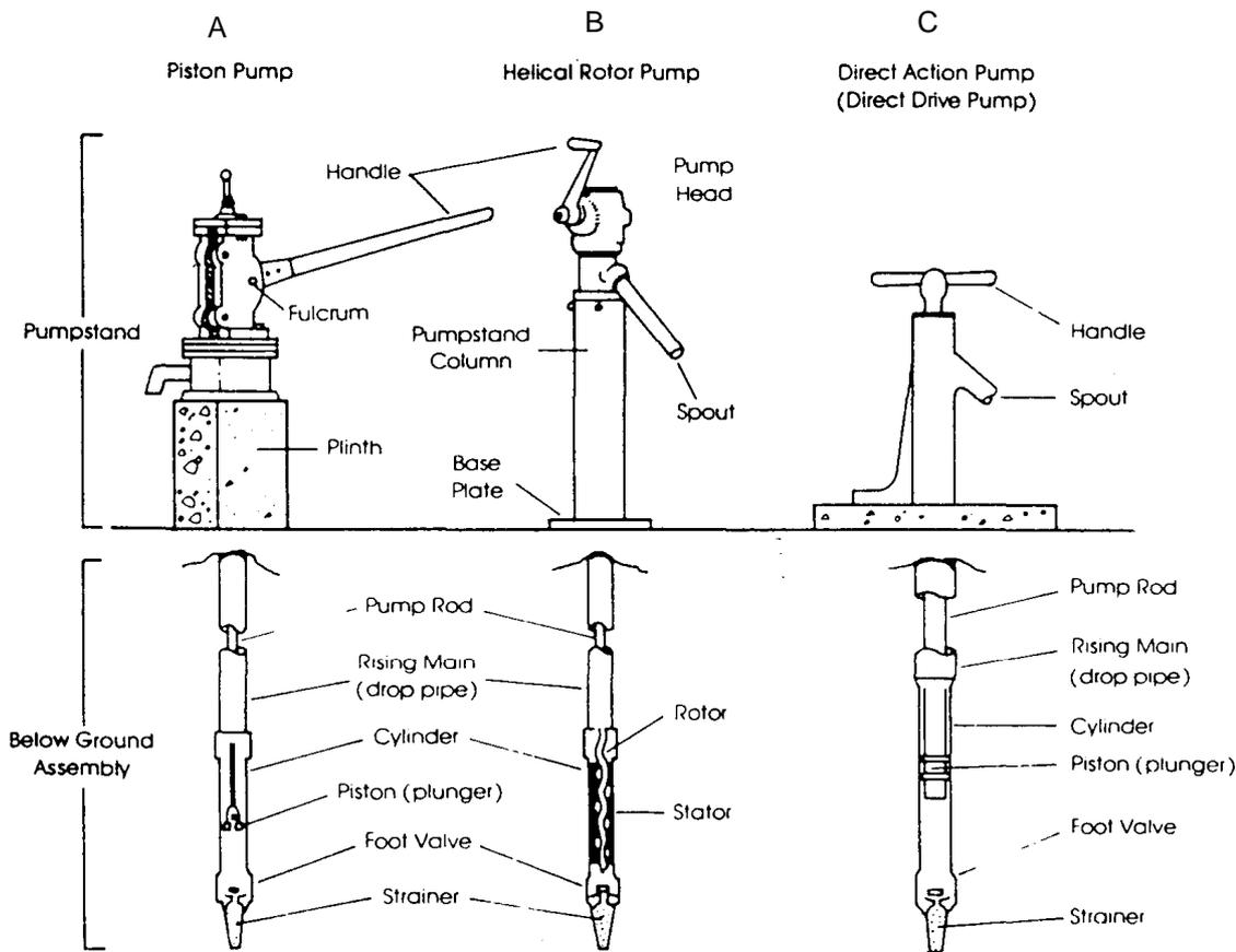
Figure 6: Types of deep-well pumps – deep-well piston, helical rotor and direct action
