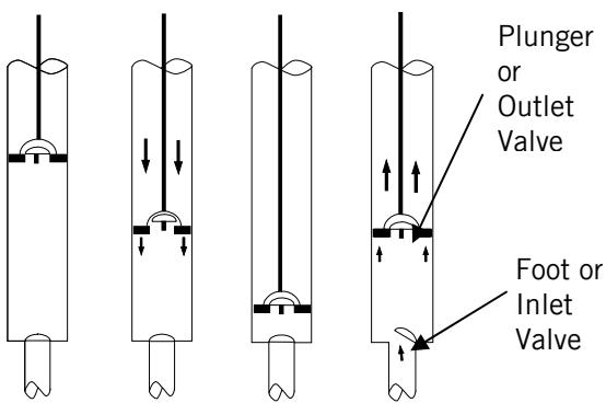
Figure 2: How most types of pump cylinders work.
