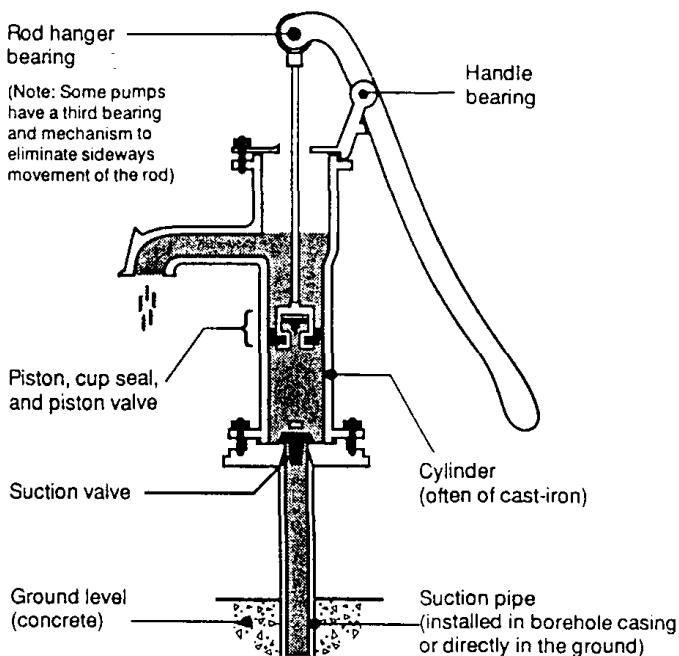
Figure 3: Shallow-well piston pump
