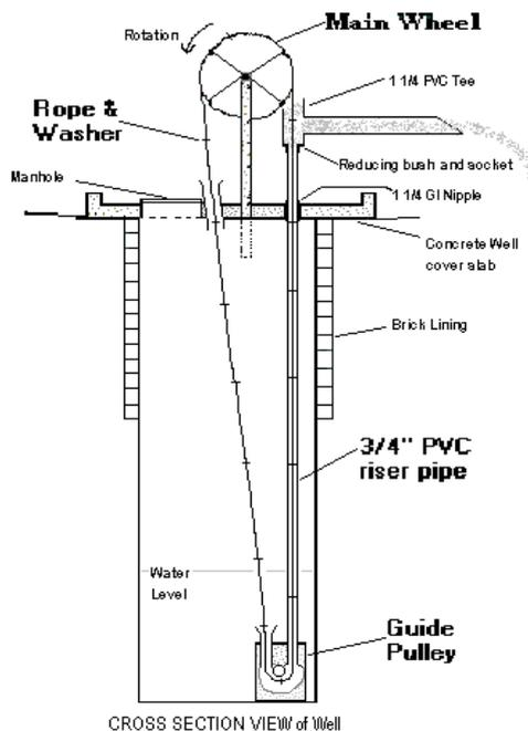
Figure 7: Rope and washer pump.
