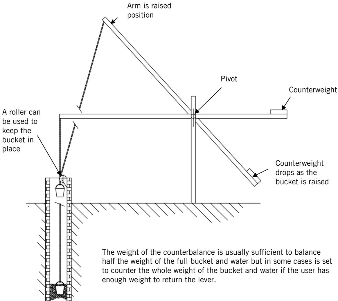
Figure 1: A counterpoise lifting device, also known as a shadouf, over an open well. A counterbalance helps lift the bucket of water.
