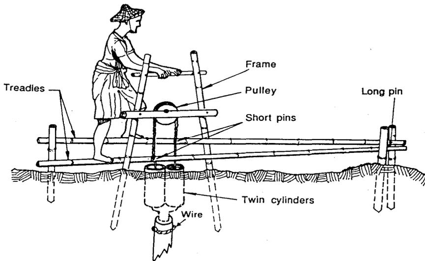
Figure 5: Treadle pump
