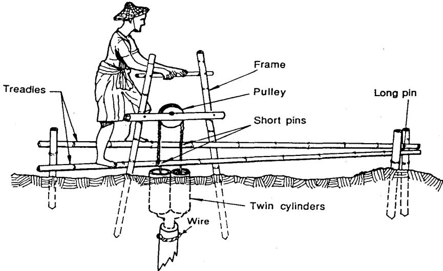
Figure 5: Treadle pump
