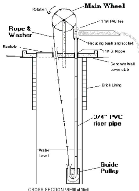
Figure 7: Rope and washer pump.
