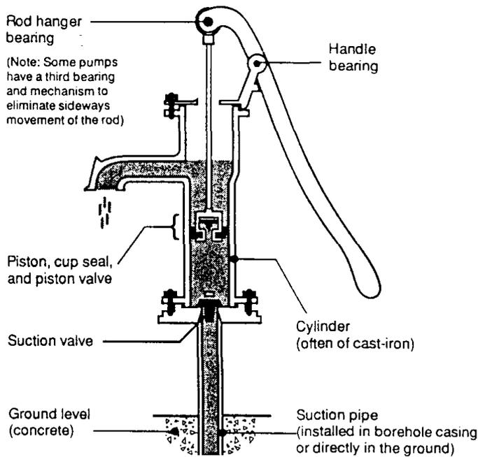
Figure 3: Shallow-well piston pump
