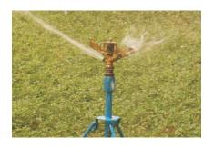
iii) Impact Sprinkler: It is made of metal or plastic and has a spring which makes the hammer move, rotating the sprinkler. It covers an area with a radius of 10-12 meters and operating pressure required is 10-20 meters.
