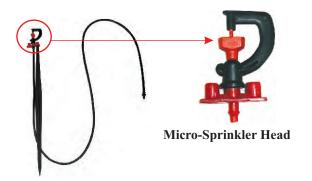
i) Micro-Sprinkler: It has a small rotating device to spray water as light precipitation. It covers an area with radius of 3-4 meters. Operating pressure required is 5-10 meters.
