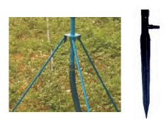
vi) Stakes/Tripod stand: Micro sprinklers and mini sprinklers are mounted on 12-inch or 18inch long plastic stakes and connected to the lateral pipes through an extension pipe. Impact sprinklers are mounted on a metal tripod stand.
