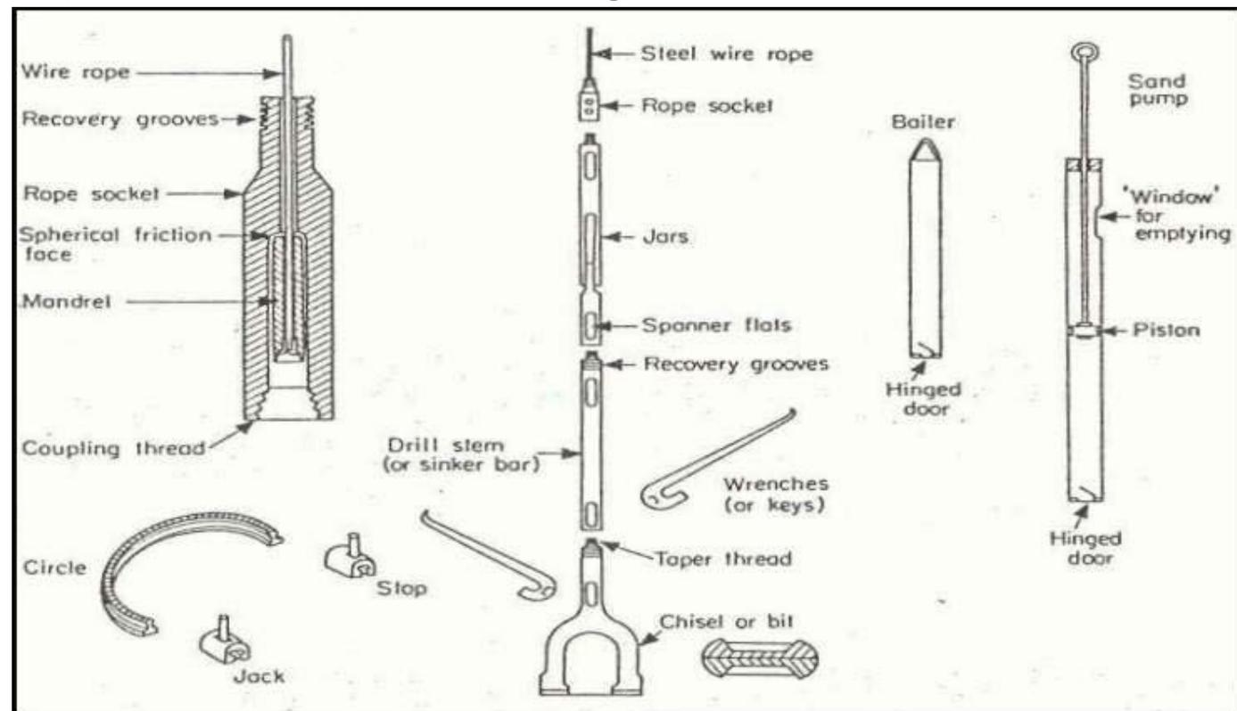
**Figure 5.6:** Cable tool or percussion drilling tools
