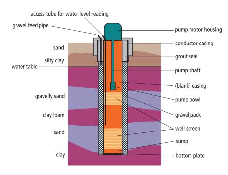
Figure 1. Components of a well.
