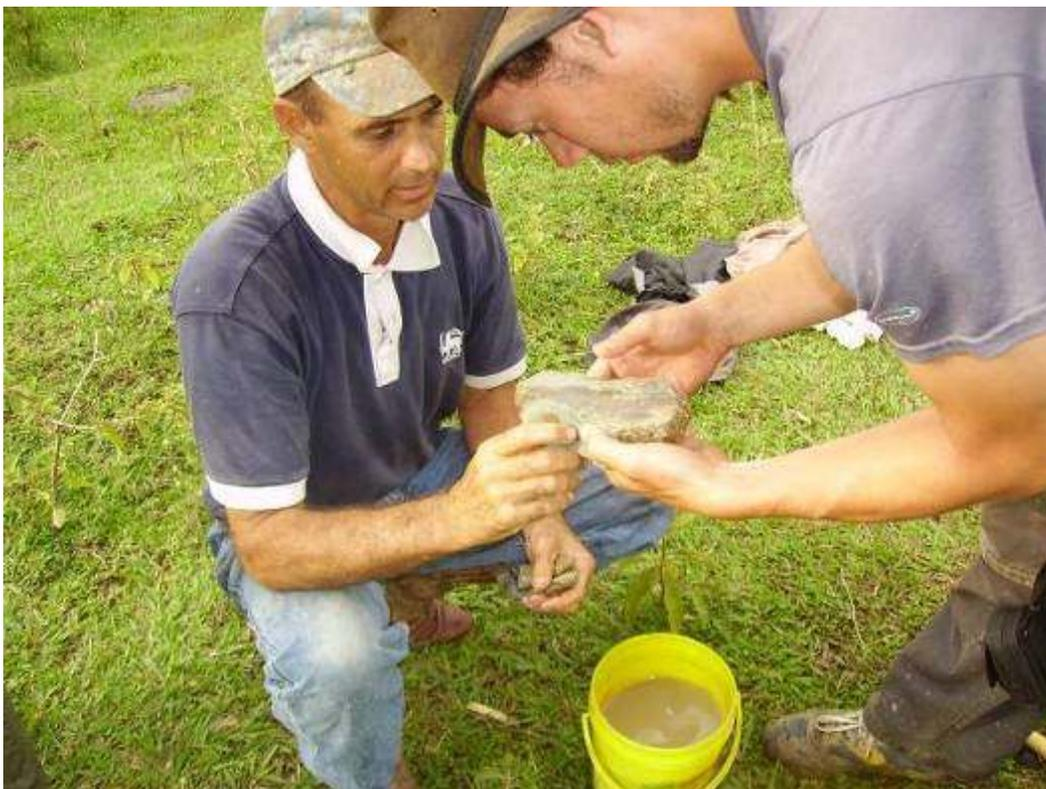
A hydrology student and myself examine metamorphic sedimentary rock from the hole and rock formation that was drilled through. It broke off in smooth sheets. We avoid this hard rock when we can. But we did pass through about a several feet of it in a couple of hours..
