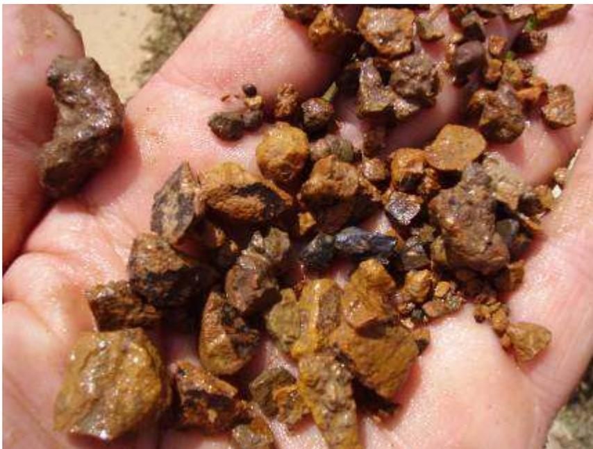
Cuttings reoved from settling pit showing what material was drilled.
