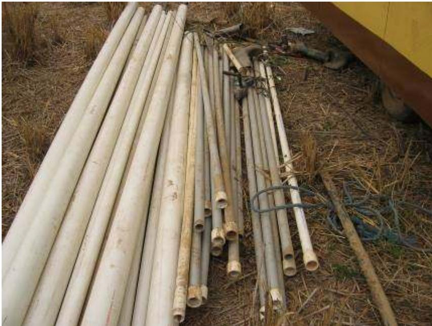
Some typical Baptist plastic PVC Drill stem and standard class 9 well casing. This drill stem is 1.25 inch schedule 40 with threaded ends with plastic couplings.
