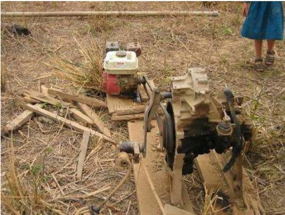
Home made adaptation for motorizing Baptist drill method. Note the 3 meter length of plastic drill stem in back ground.
