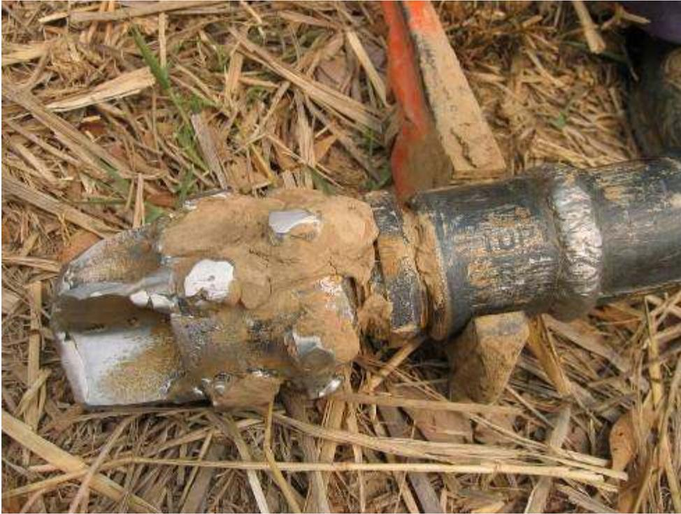
The home made drill bit coupled to typical 1.25 inch metal drill pipe. (we use many types of bits) The driller reported he used 12 meters of drill pipe for the deep wells in this area. We usually use only 6 meters for wells to the 50 meter range. The driller report he had to pass through two thin layers of soft rock. The driller reported his 105 meter deep well took a 5 days to drill using his home made motorized adaptation to pull
