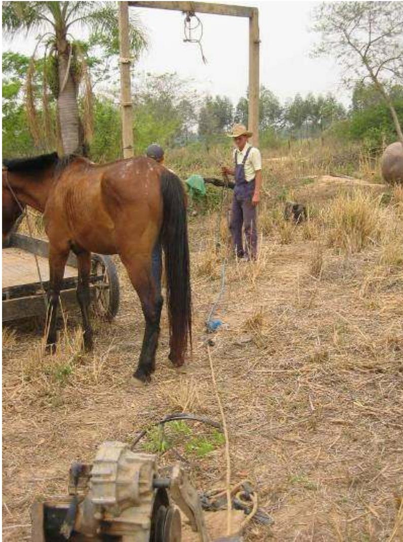
Typical Baptist Drilling technique “arco” cross bar shown with rope rigged to be pulled by home made motor adaptor. adaptation. Instead of people.
