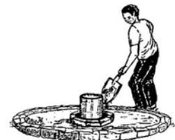
Pour the concrete slab and form the protective collar.
